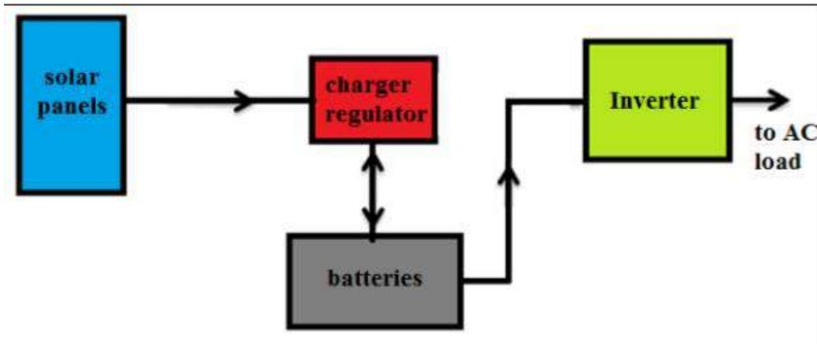
Figure (3-31) The connection of the solar system with the simple inverter
