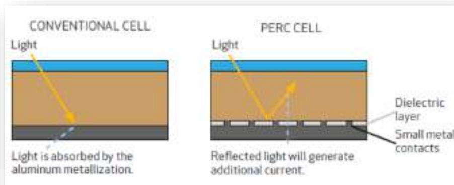
Figure (3-13) perc cell
