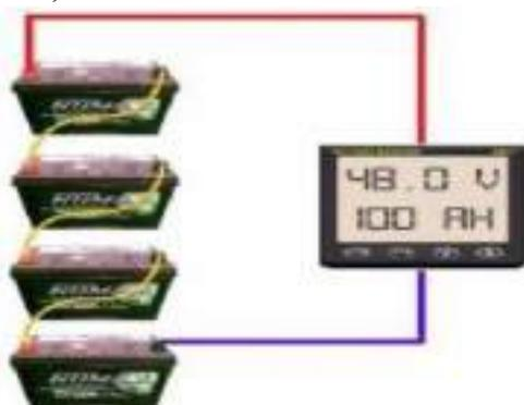
Figure (3-34) Series connection of batteries
