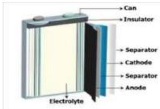
**Figure (3-33) Lithium-ion battery**
