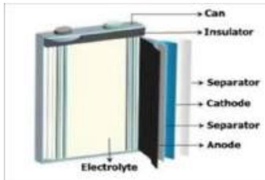
**Figure (3-33) Lithium-ion battery**
