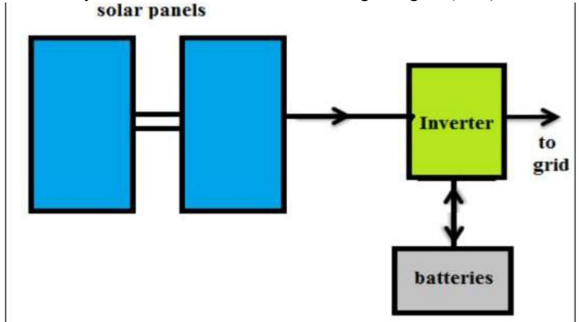
**Figure (3-29) The connection of the solar system with the inverter/charger**
