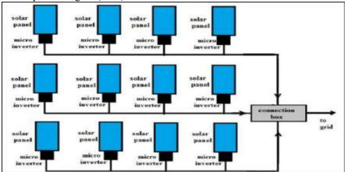
Figure (3-25) The connection of the solar system with microinvert
