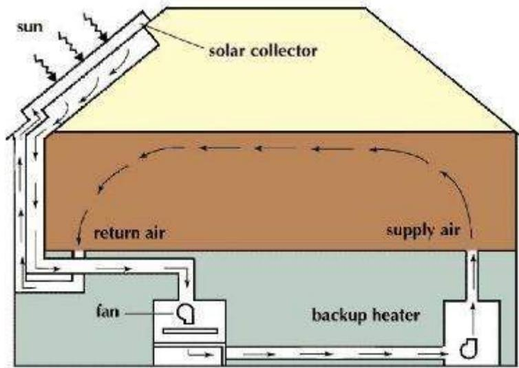
**Figure (2 – 6) Solar Hot Air Systems**
