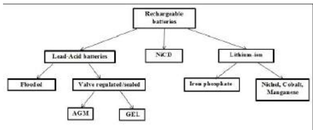
Figure (3-32) The different types of solar batteries
