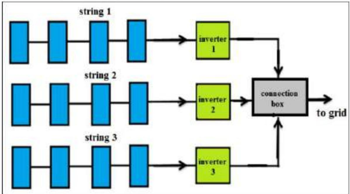
**Figure (3-21) Solar system connection with the string inverter**
