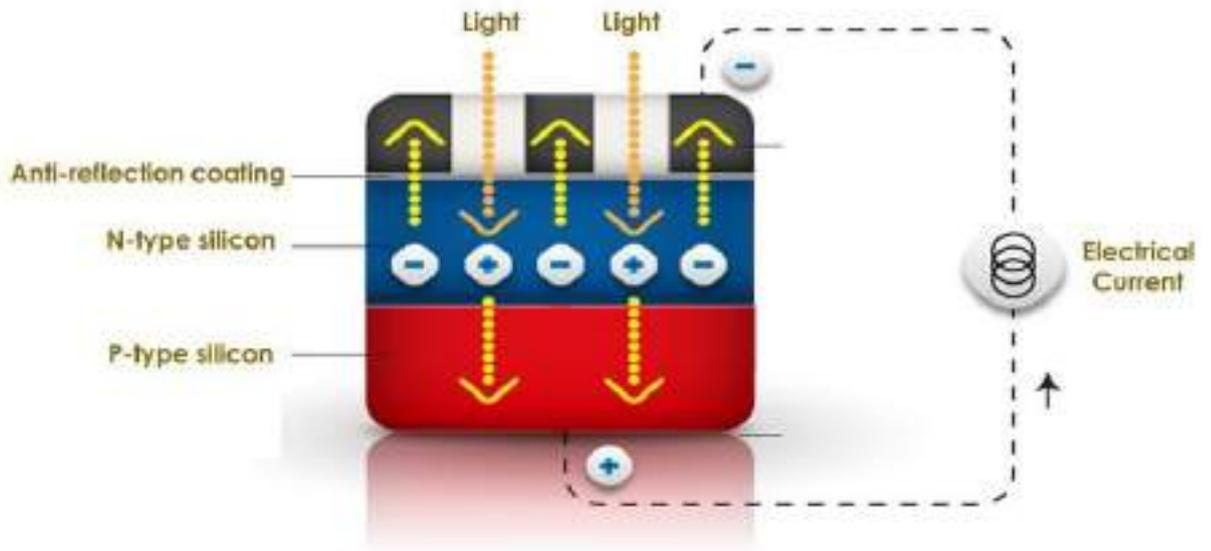
**Figure (3- 2) how do the solar cells work**
