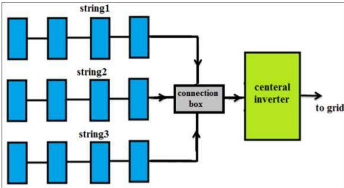
**Figure (3-17) The connection of the solar panel to the central inverter**
