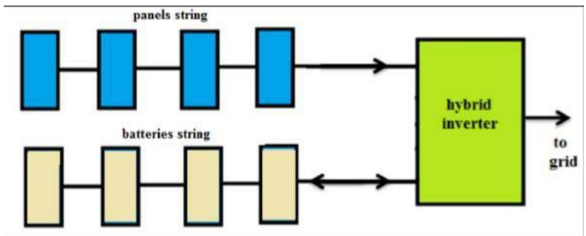
**Figure (3-27) The connection of the solar system with hybrid inverter**
