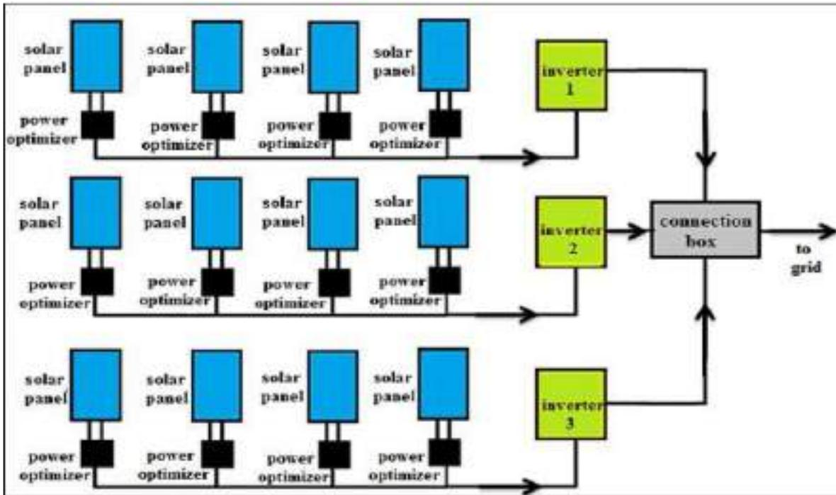
**Figure (3-23) The connection of the solar system with power optimizer devices.**
