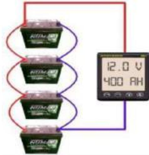
**Figure (3-35) Parallel connection of batteries**
