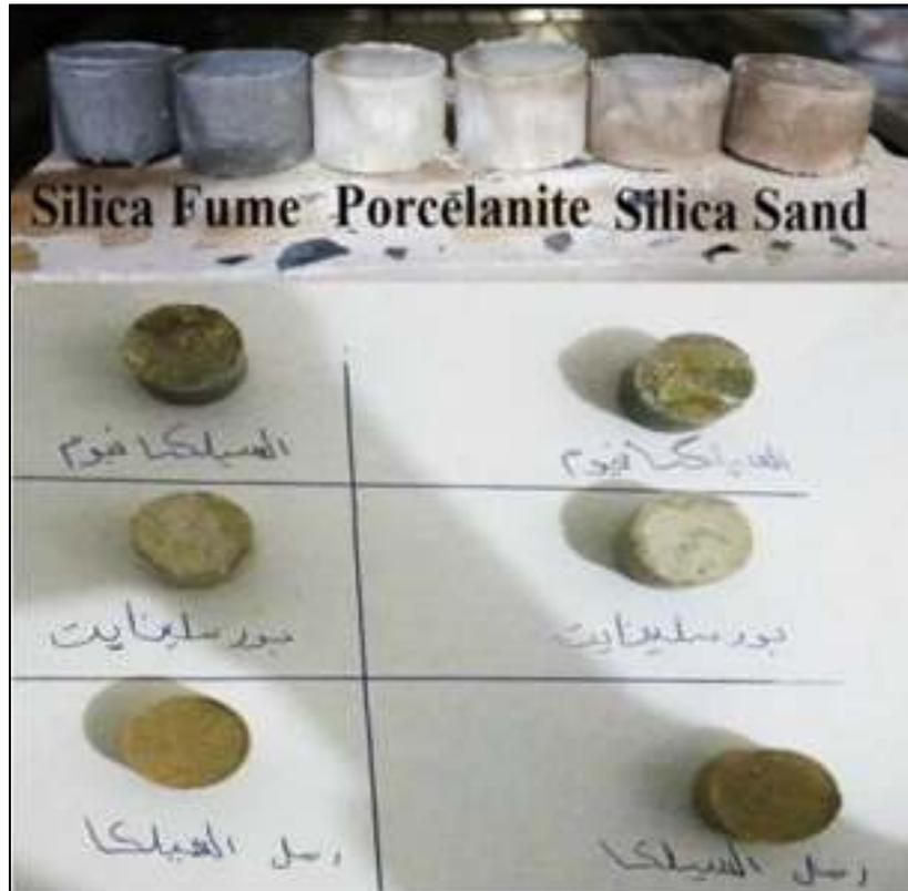
Figure (3-3) The samples after firing
