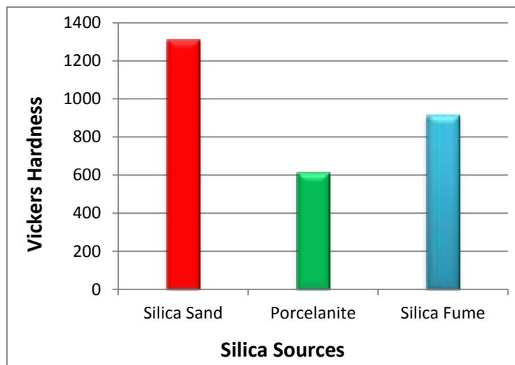
Figure (4-5) Hardness of the porcelain samples with various sources of silica.
