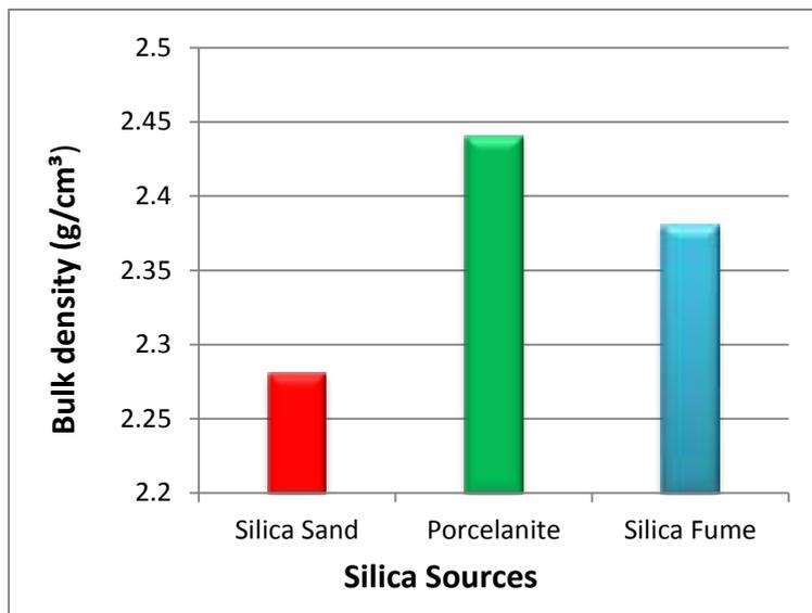
Figure (4-3) The bulk density of porcelain samples with various sources of silica.
