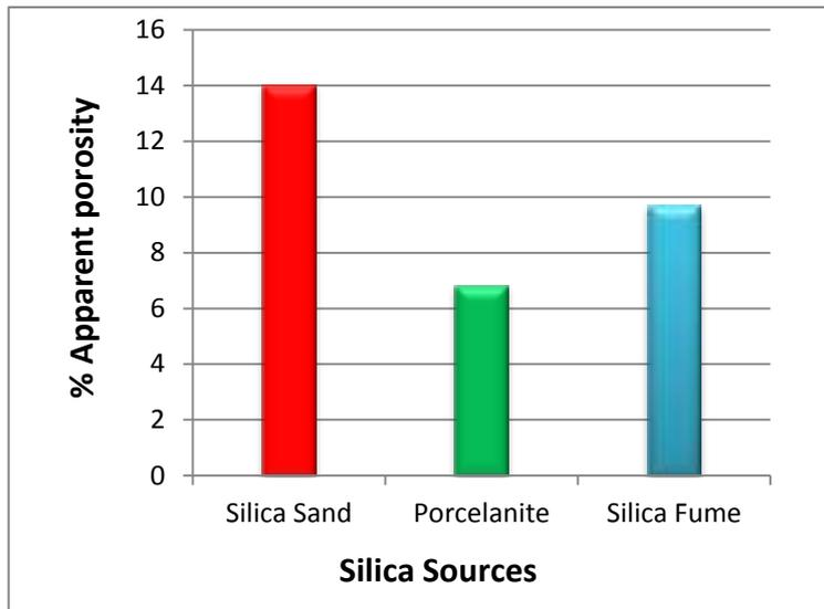
Figure (4-2) The apparent porosity of porcelain samples with various sources of silica.
