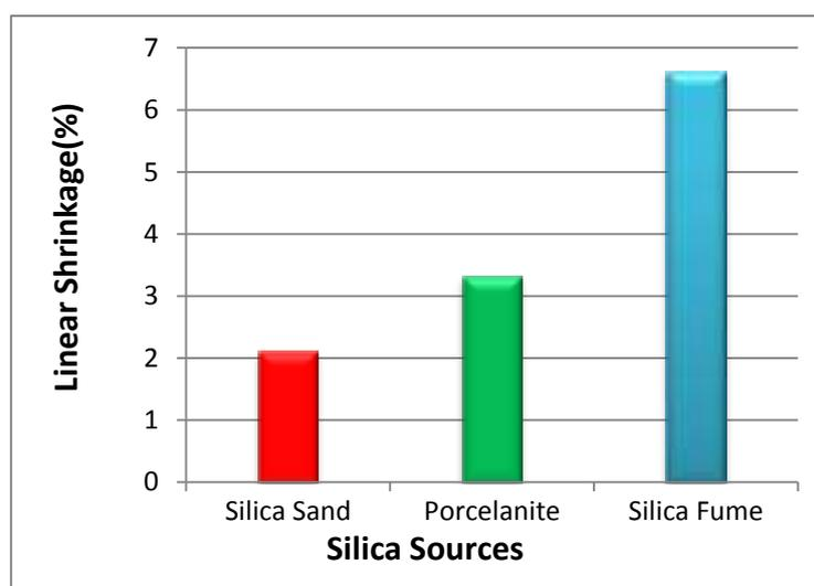
Figure (4-1) Linear shrinkage of porcelain samples with various sources of silica.
