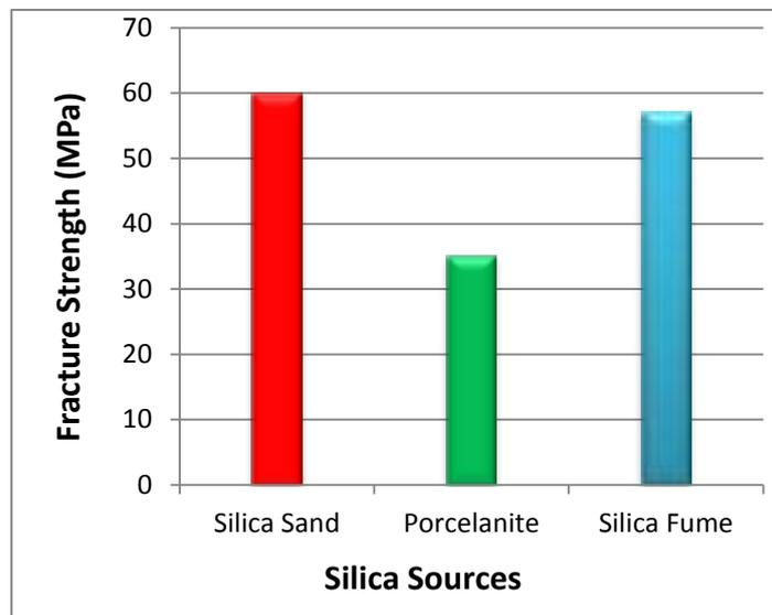
Figure (4-4) Fracture strength of the porcelain samples with various sources of silica.
