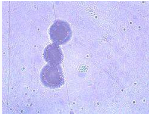
Lycopodium club moss spores (diameter about 60 micrometers) captured on an electrospun polyvinyl alcohol fiber
