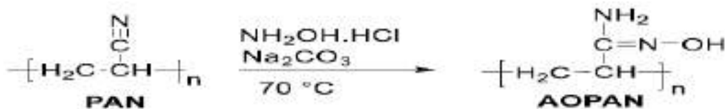
Scheme.1 Reaction of hydroxylamine hydrochloride with PAN nitrile group
