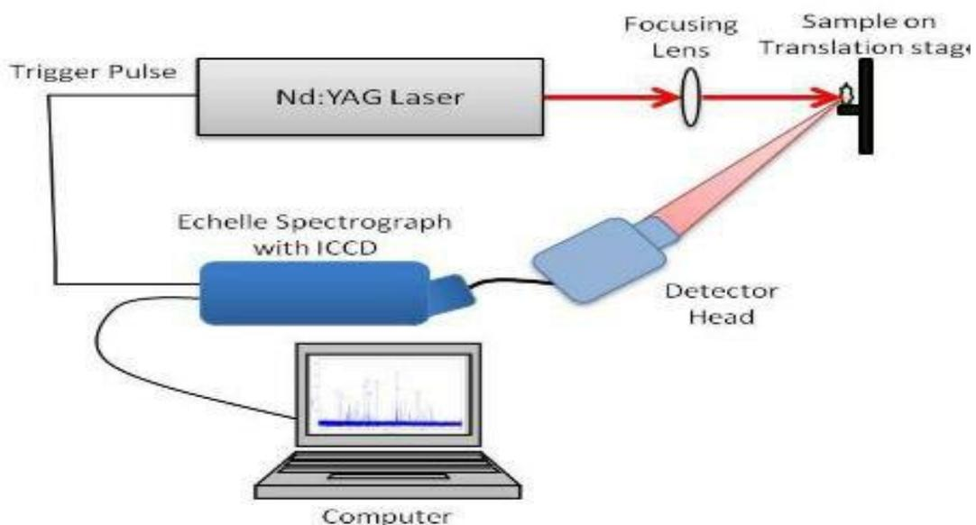
**Figure 2** LIBS set-up used for the current study
