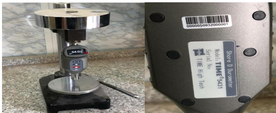
Figure(3-4) : Diagram showing the Hardness test device
