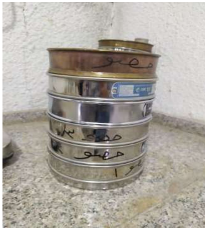
Figure (5) shows the sieves used in the grading of the aggregate
