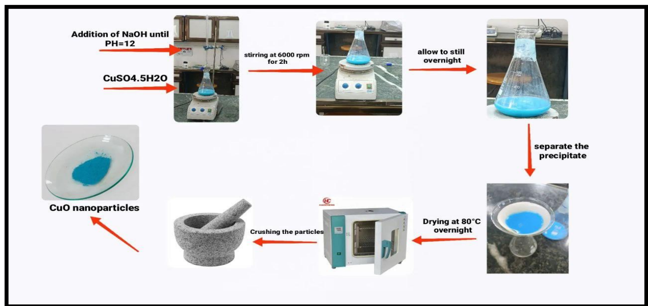
Figure 2-1: Schematic Diagram of the steps used for synthesizing CuO NPs.
