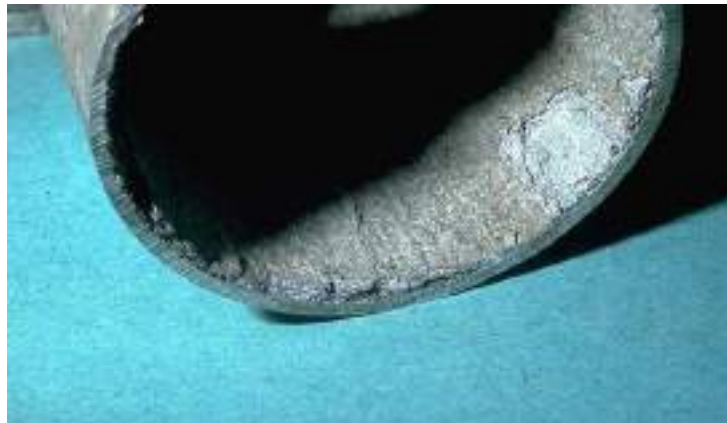
Fig. (2-6) Intergranular corrosion of metal [26].
