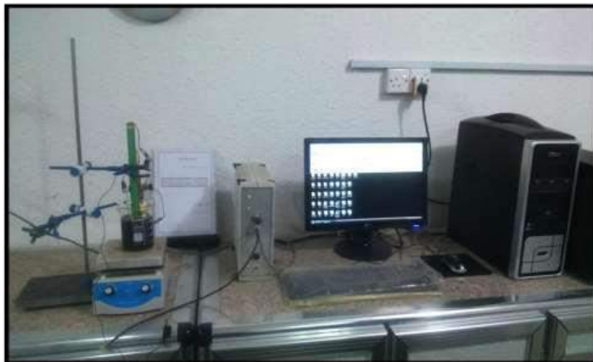
Fig. (3-5) Potentiostatic test in an inhibitor
