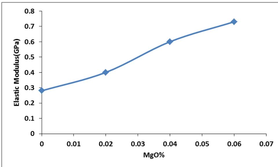
**Figure (4-4) Elastic Modulus for Blend (PVA/PEG) and Nanocomposite as a Function of Different Percent of MgO Nanoparticles**
