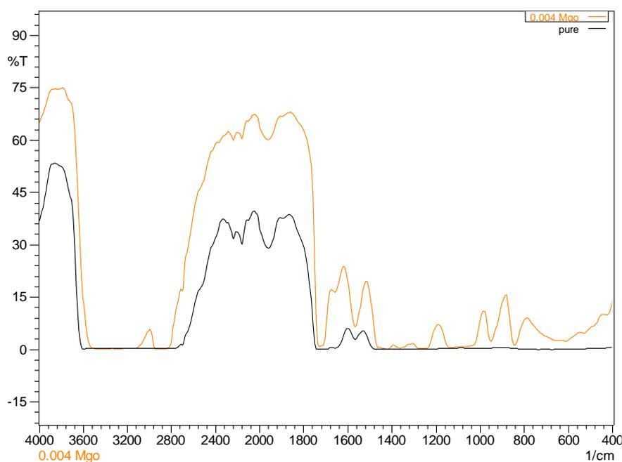
**Figure (4-1) FTIR Spectrum of blend (70%PVA+30%PEG) & Nanocomposite Materials (70%PVA+30%PEG+ 0.4% ZnO).**
