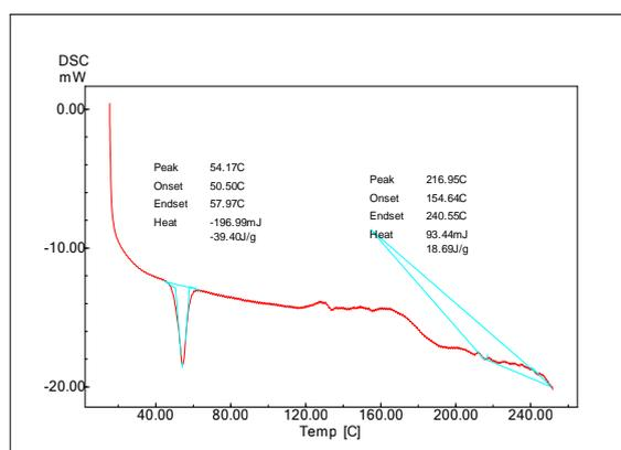
**Figure (4-2) DSC for Melting Endotherm and in Nitrogen Atmosphere A- Blend PVA/PEG, B- PVA/PEG/0.2%MgO, C- PVA/PEG/0.4%MgO, and PVA/PEG/0.6%MgO**
