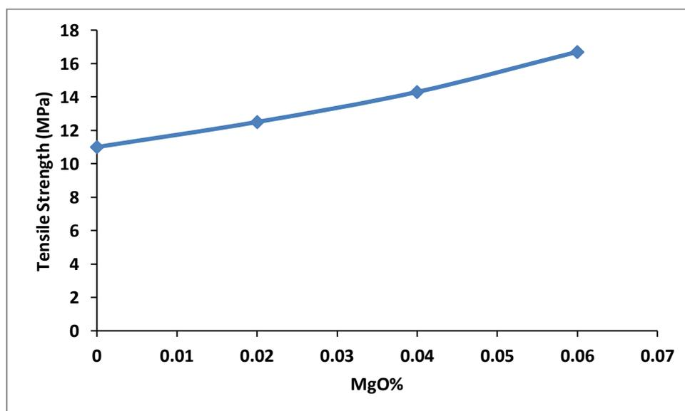
**Figure (4-3) Tensile Strength for Blend (PVA/PEG) and Nanocomposite as a Function of Different Percent of MgO Nanoparticles**
