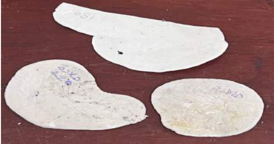
Figure (4.9): it Show the sheets of LDPE 45g+5g zno
