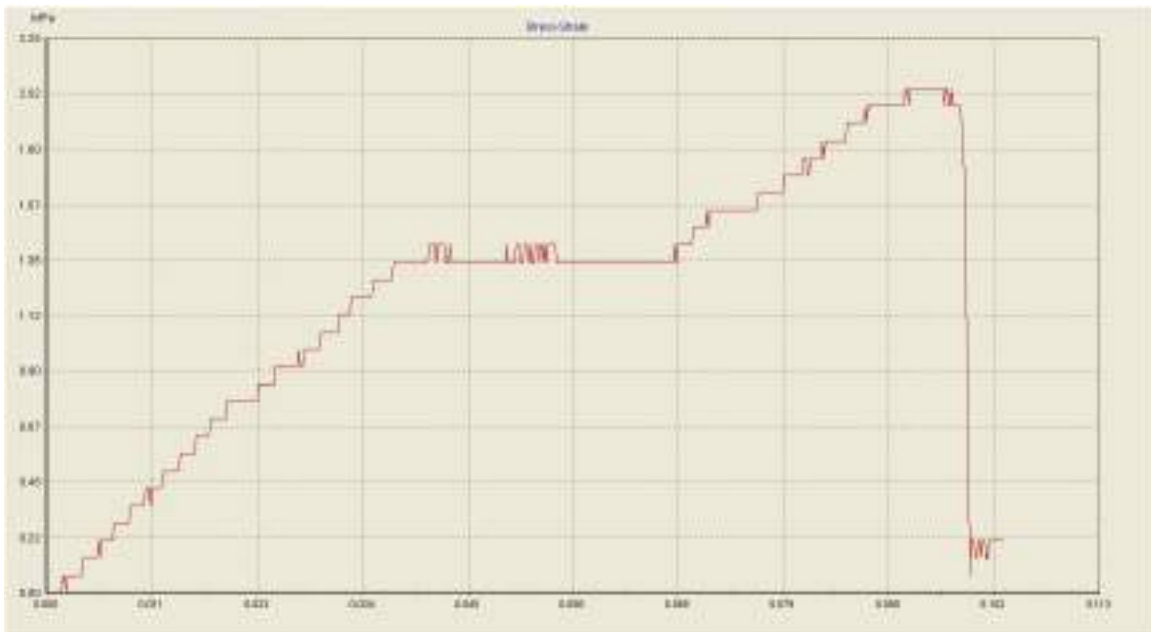
Figure (4.3): It Shows a stress-strain diagram for a sample (A3).
