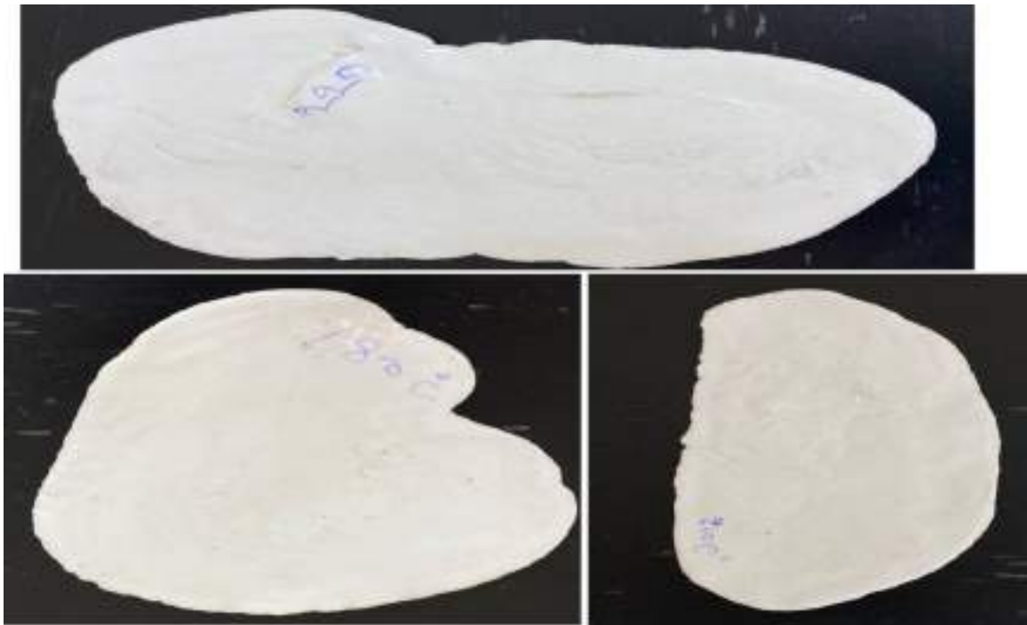
Figure (4.10): it Show the sheets of LDPE 40g + 10g zno
