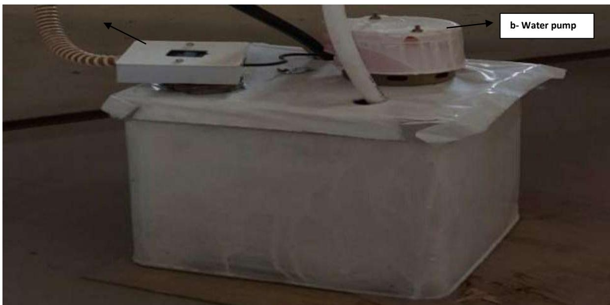
**Fig.3-5: Coolant tank**
