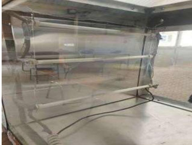
**Fig.3-9: The electric heater**
