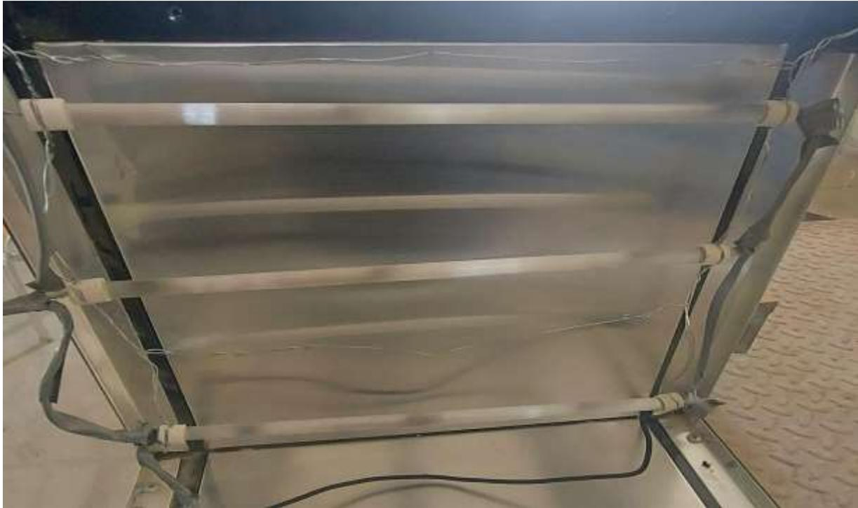
**Fig.3-4: The electric heater**
