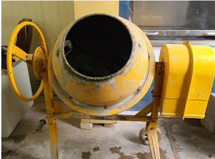
Figure (3.3) The mechanical mixing
