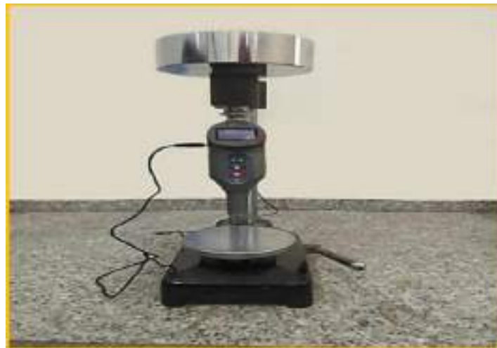
Fig. 2. 3. The hardness test device using (shore D)
