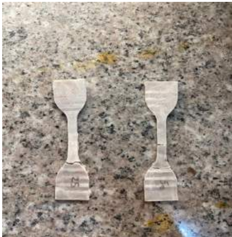
Fig. 2.8. Tensile test sample before and after measurement.
