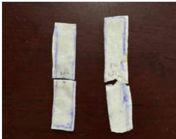
Figure (2.10): Impact test sample before and after measurement.
