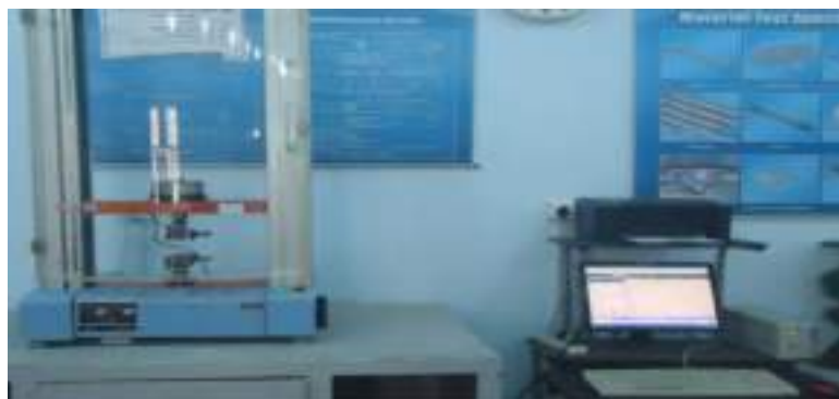
Fig. 2. 2. The tensile test device
