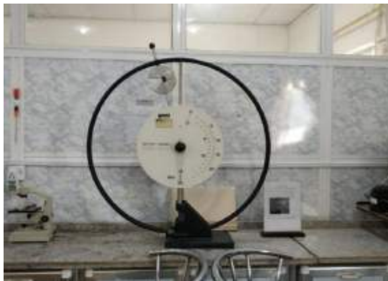
Fig. 2. 4. The impact test device by a charpy method
