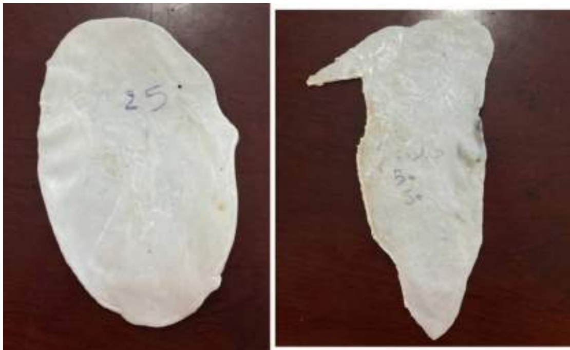
Figure (2.9): it Shaow the sheets of pure PET+PP for hardness test.
