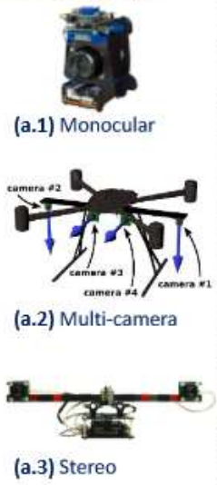
Figure 6. Classes of vision system and examples of configurations (location and orientation)
