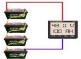
Figure (3-34) Series connection of batteries
