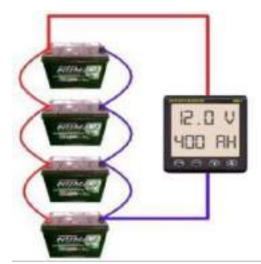
**Figure (3-35) Parallel connection of batteries**
