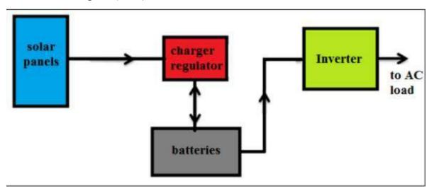
Figure (3-31) The connection of the solar system with the simple inverter
