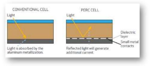
Figure (3-13) perc cell
