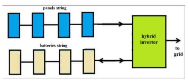
Figure (3-27) The connection of the solar system with hybrid inverter
