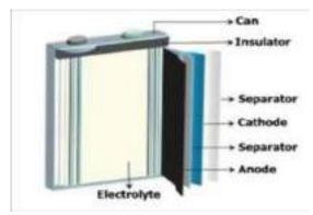
Figure (3-33) Lithium-ion battery
