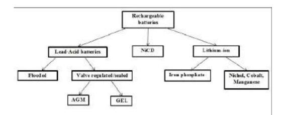
Figure (3-32) The different types of solar batteries
