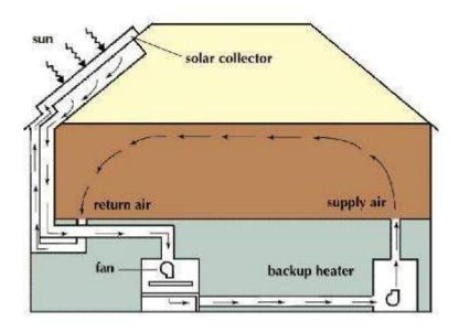
Figure (2 – 6) Solar Hot Air Systems
