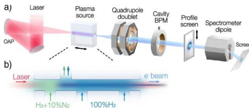
**Fig 1.3: Laser-plasma accelerator. (a) Schematic LUX laser and electron beam line.**
