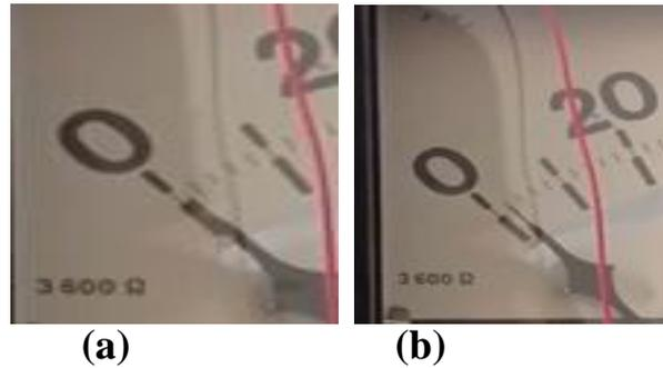
**Fig 3.2: Current increasing with laser pulses, (a) shows the electron current when laser intensity equals to zero, there is no change in current, where the current here equals to 0.5  $\mu$ A. (b) shows the current with a laser pulse of intensity of 500 mw, the current has increased to 1  $\mu$ A.**
