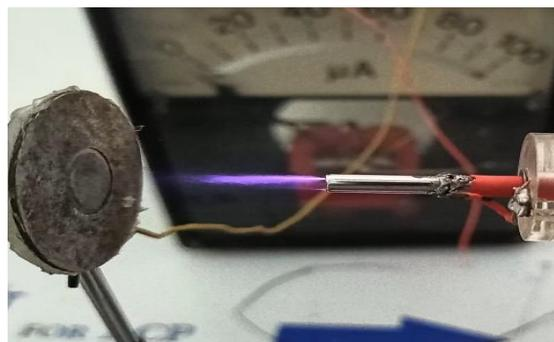
**Fig 2.2: A photograph for the plasma jet system**
