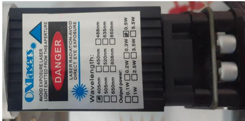
**Fig 2.3: The laser used of 500 mW output and 405 nm wavelength.**
