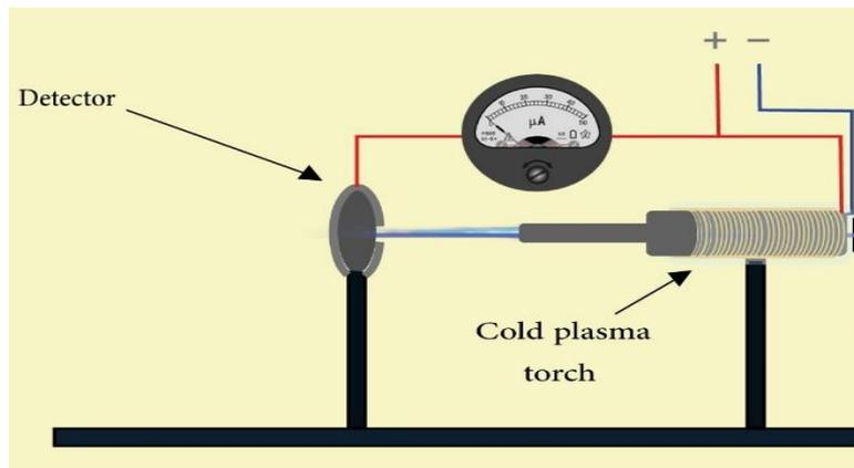
**Fig 2.1: The plasma jet system scheme.**
