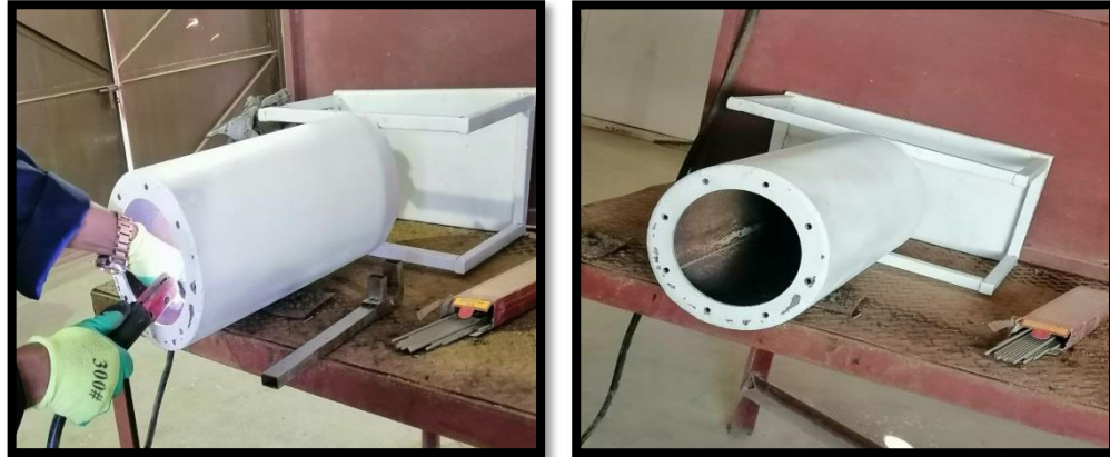
Figure (3-2) The iron rod and the base after the cleaning process
