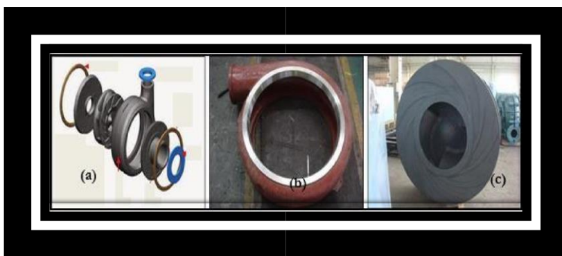
FIGURE 1 Slurry pumping components consisting of HCWCI
