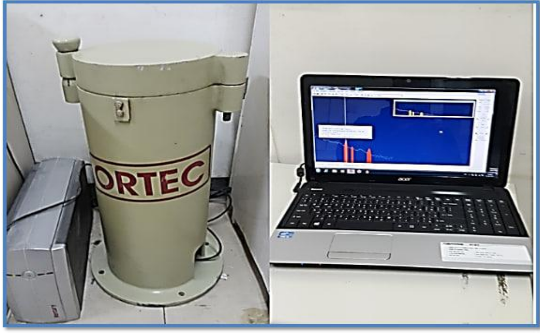
Figure(3.3): The gamma spectrum recorded using the MAESTRO-32 Software
