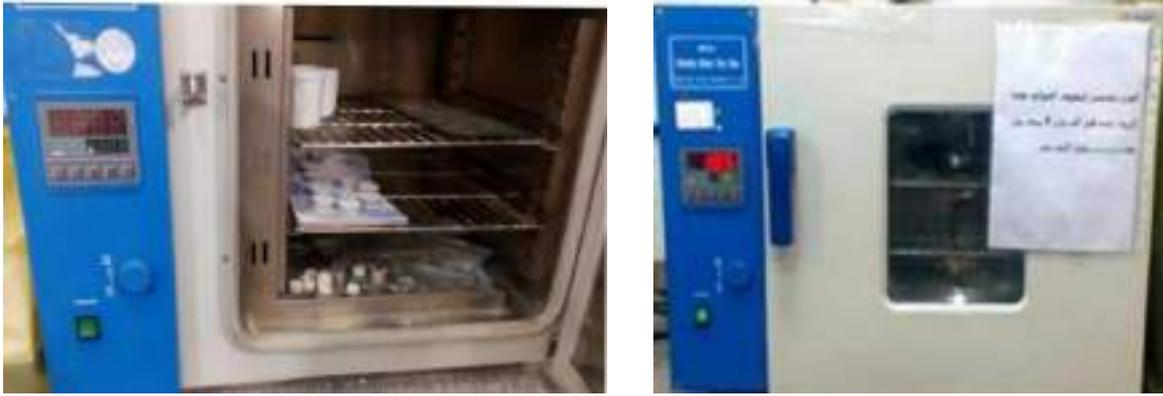
**Figure (3-4) Drying oven**
