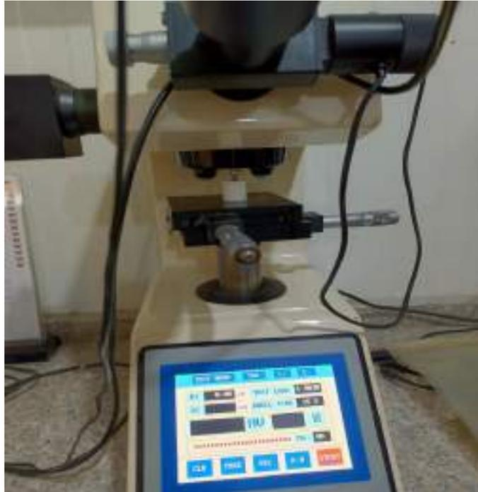
**Figure (3-8) Microhardness device**
