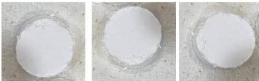
**Figure (3-5) samples after sintering**
