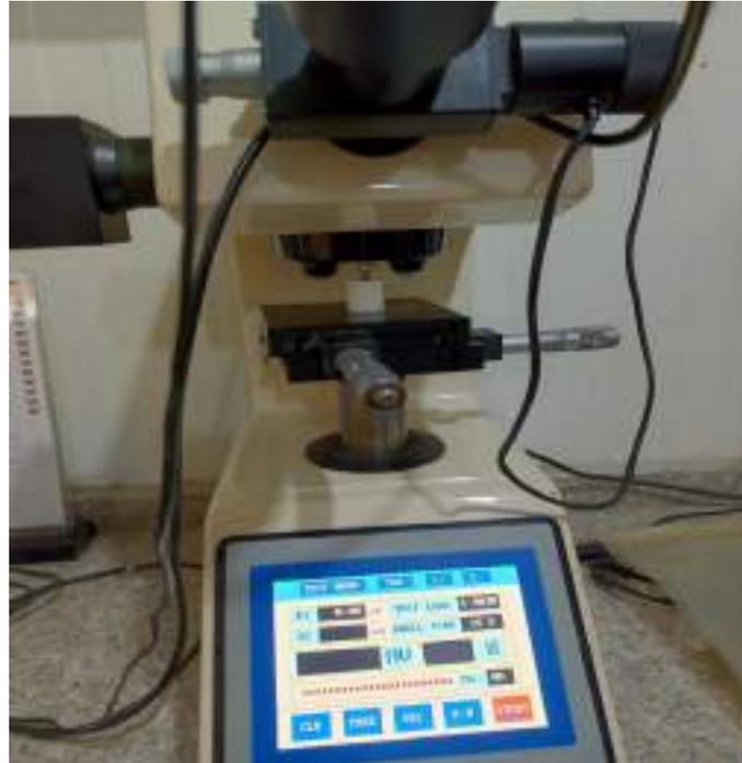
**Figure (3-8) Microhardness device**
