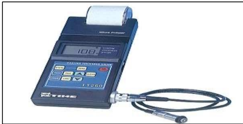
Fig. (3.5): Shows the device of thickness measuring.
