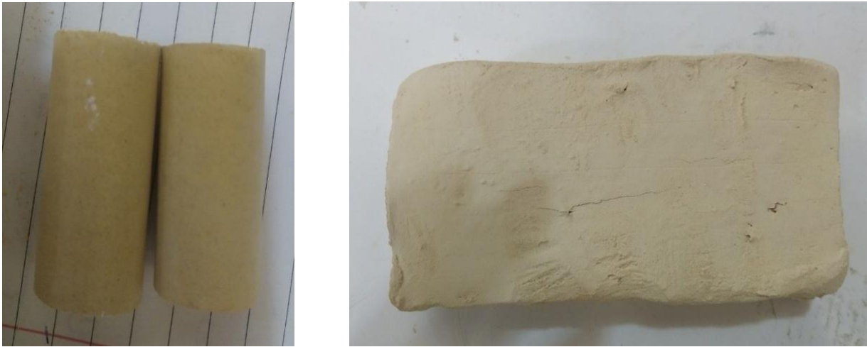
Figure (3-6:) The pressed and extruded samples after firing
