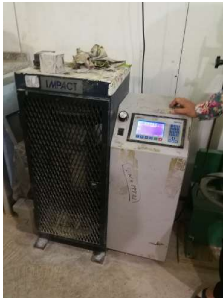
Figure (3-6) : Compressive strength test machine and sample.
