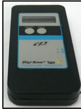
Figure 3.2. Digi-Sense 91000-00 Type K Data Logger (Thermometer 2015)
