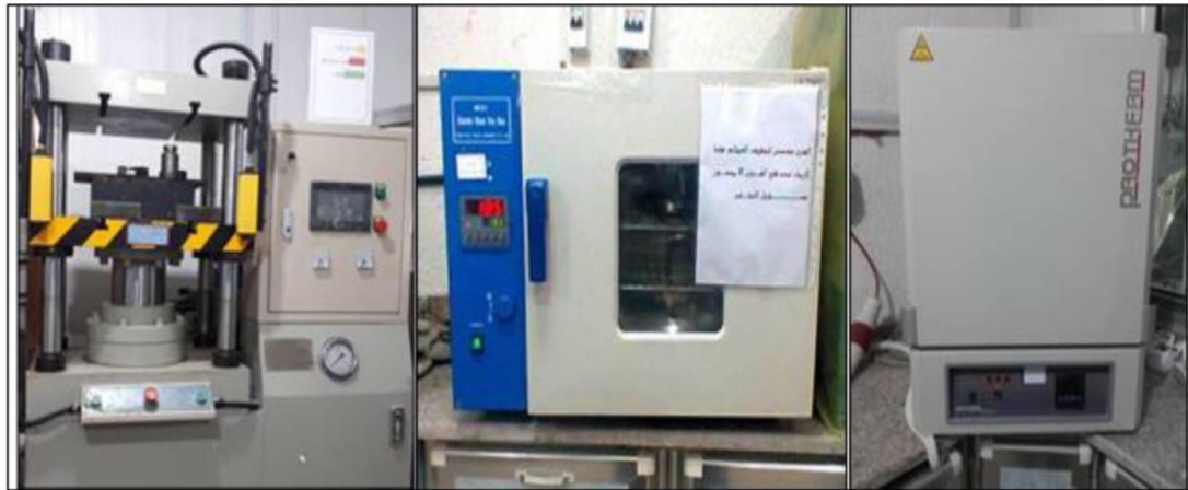
(a) (b) (c) Figure (3-2): a) Pressing machine, b) Electrical drying Oven, and c) Electrical firing furnace.
