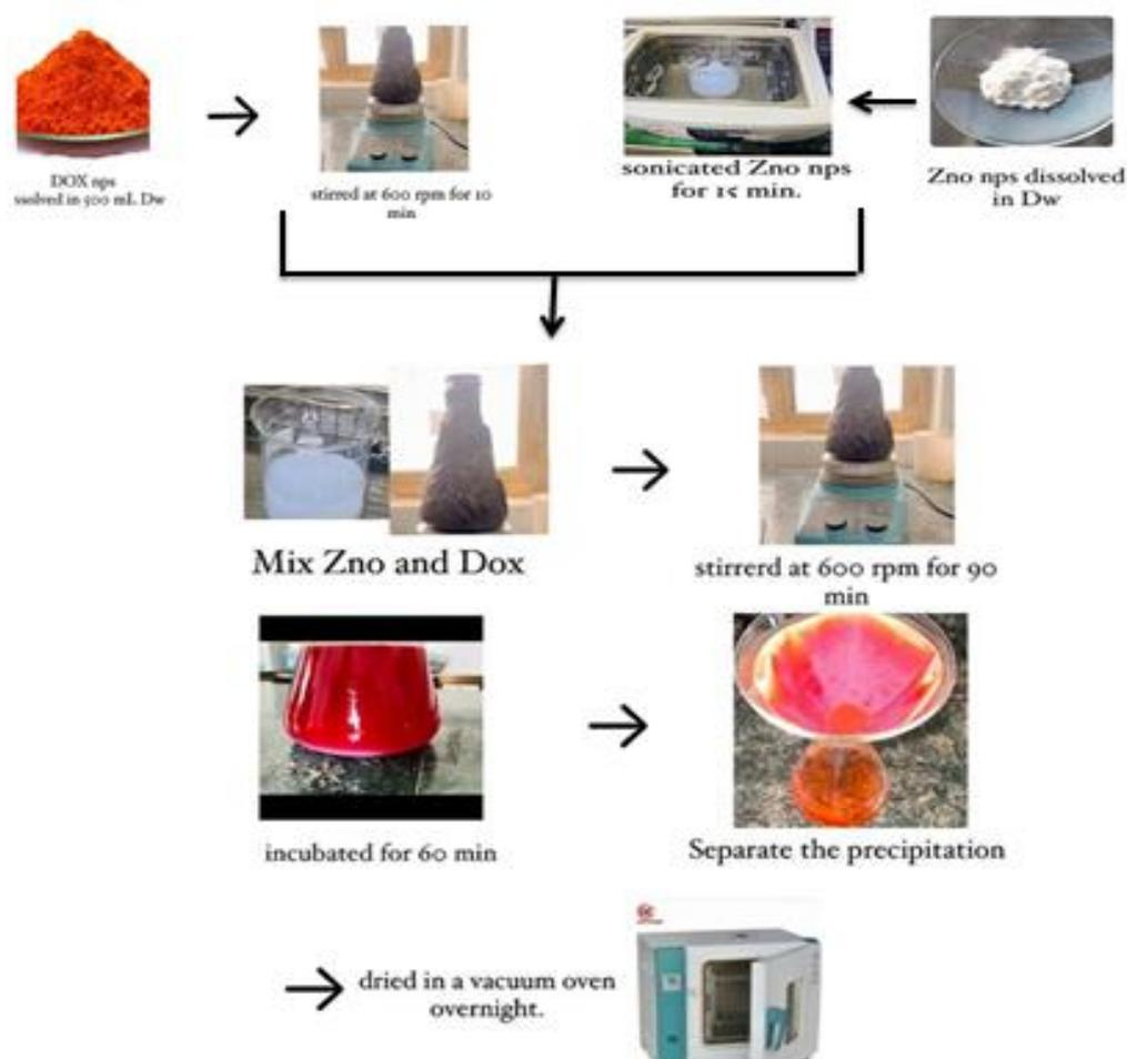
Figure (2-2): Schematic Diagram of the steps used for loading of Doxorubicin on the surface of ZnO Nano sheets.
