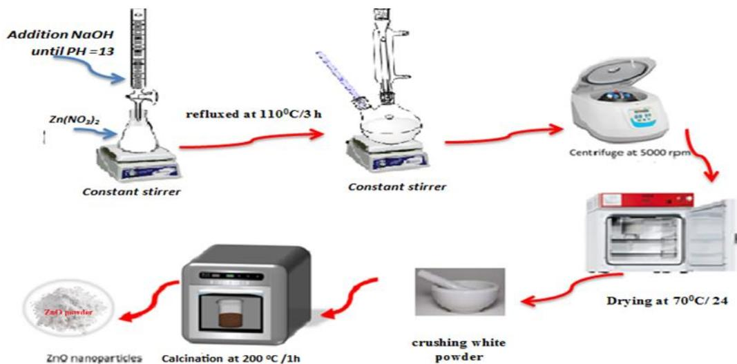
Figure (2-1): Schematic Diagram of the steps used for synthesizing ZnO nanosheets.
