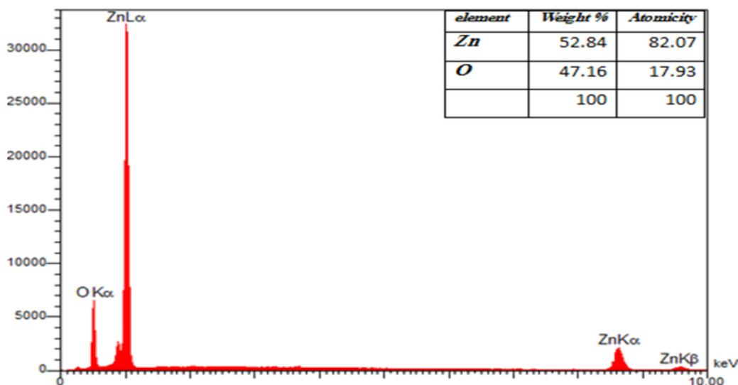
Figure (3-3): FE- SEM-EDX spectrum of ZnO nanosheets.
