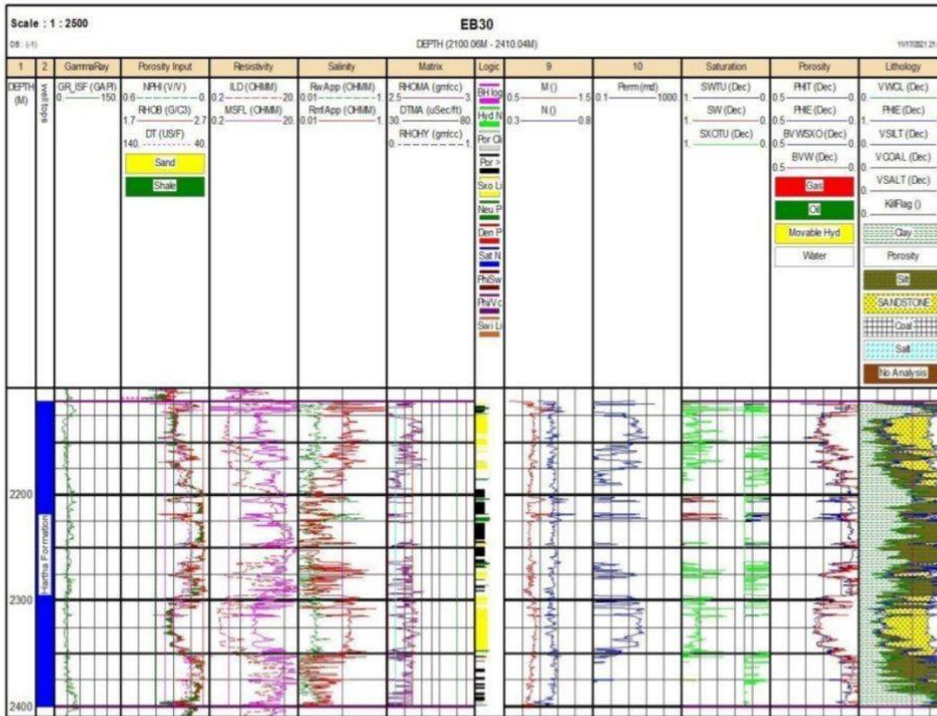
**Figure 2.3- The Computer P processing Interpretation (CPI) of the Hartha formation in well EB- 30**
