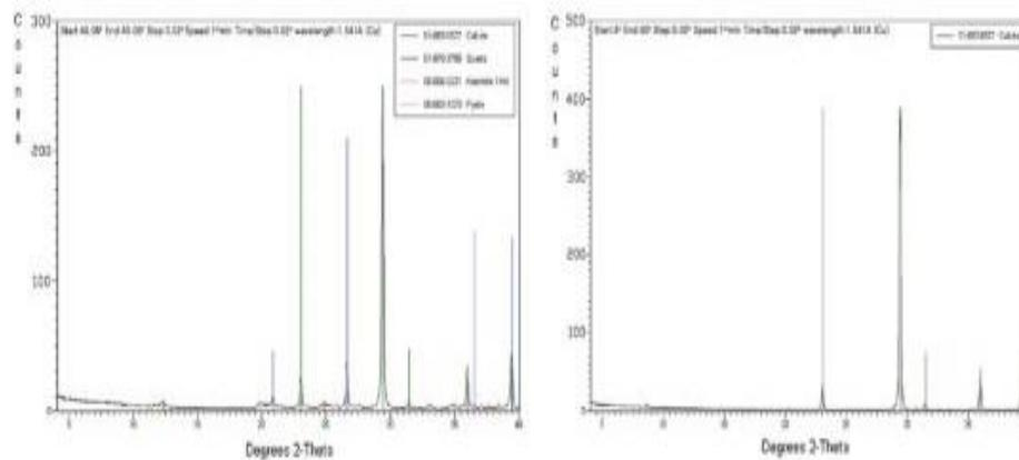
Fig. 3.2 XRD diffractograms for selected samples of the Hartha Formation
