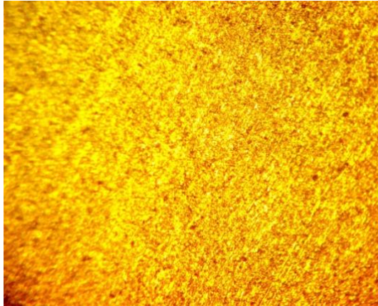
Figure (3-5) shows the microstructure of pure aluminum cast in a sand mold.
