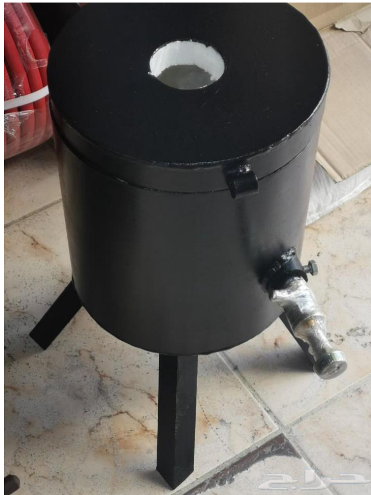
Figure (2-1) melting furnace.
