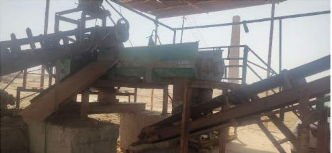
Figure.3. Ground kneader. It is a basin containing parts inside it for mixing the dirt coming from the hopper, where the clay is mixed with water to complete the kneading process to turn it into solid clay .
