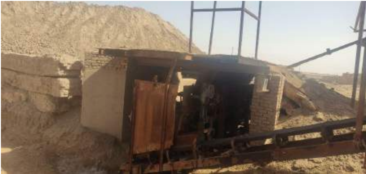
Figure.1.The hopper : It is a large basin where its work is to divide the dirt on the conveyor belt.
