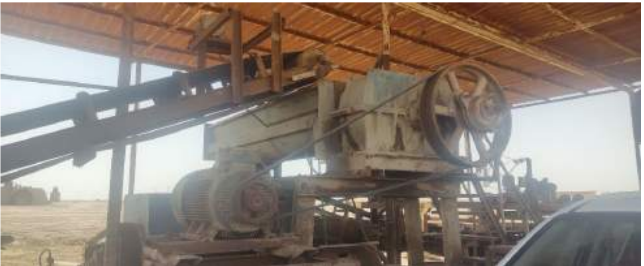
Figure.4. The upper kneader :- It is a kneader similar to the ground kneader, except that it contains a pressing chamber, the purpose of which is to empty the clay from the air.
