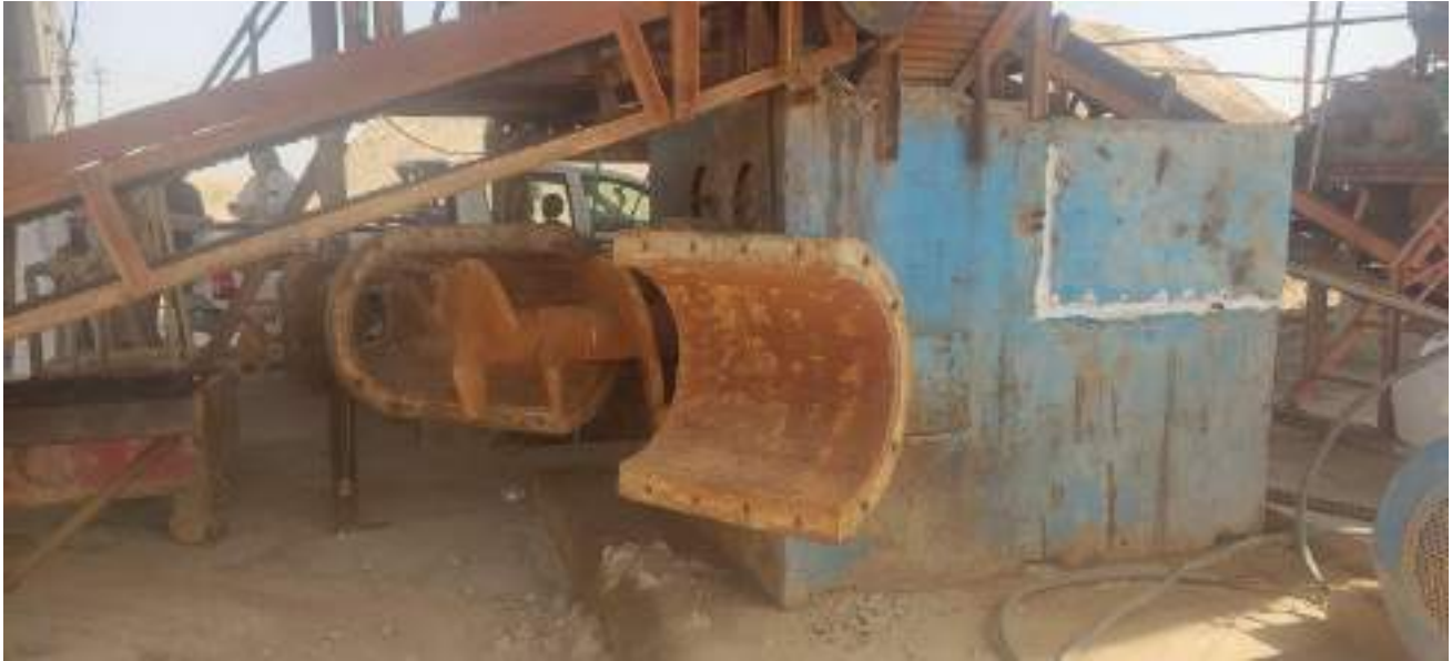
Figure.5.The machine that cuts the clay and sends it to the brick making mold.
