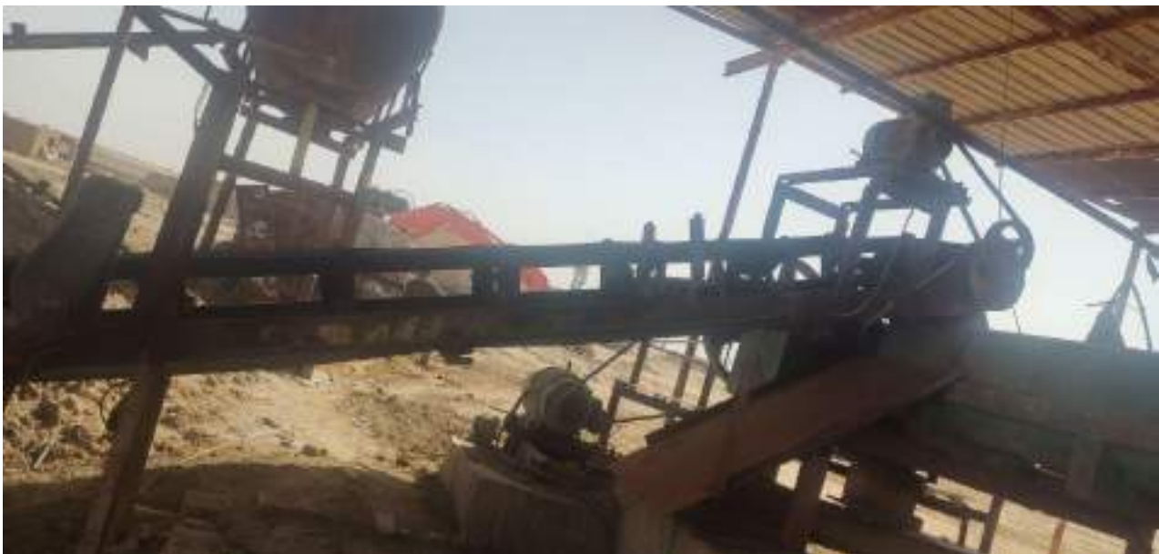
Figure.2.Conveyor belt. It is a belt that pulls the dirt from the hopper and transfers it to the kneader
