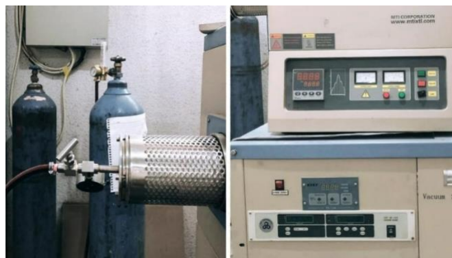
Figure (7-2) Sintering furnace
