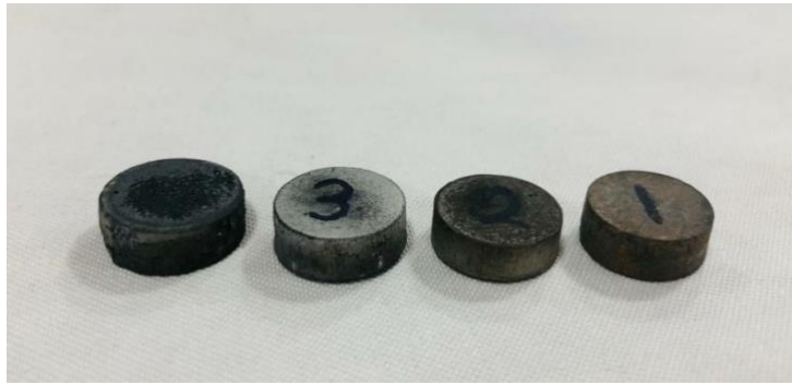
Figure (8-2) Samples after the sintering process
