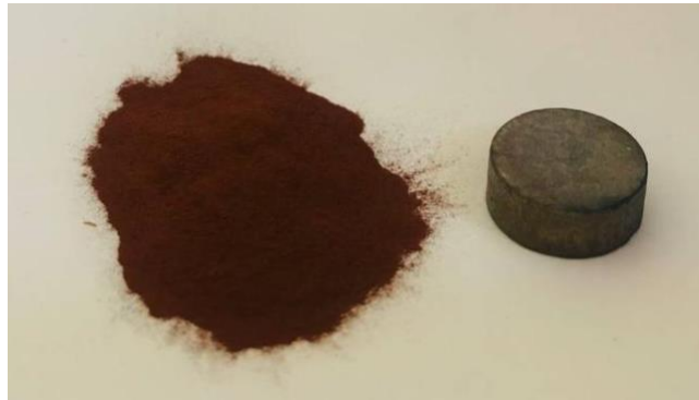
Figure (1-2) Copper metal : Powder , pressing pellet with a small percentage of zinc
