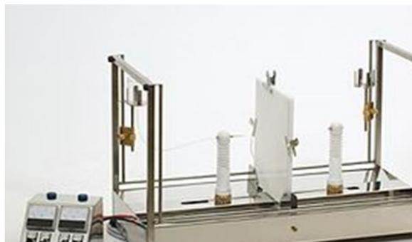
Fig.2 Apparent devise of electrospinning
