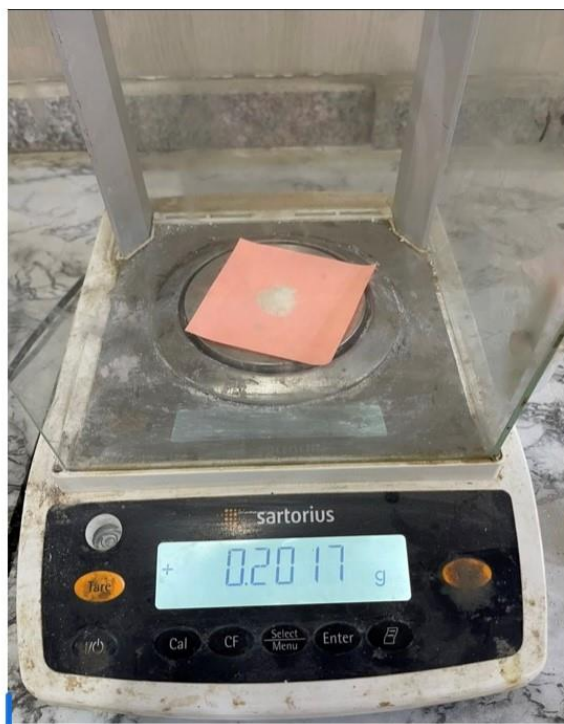
Figure 2-1. Electronic scale that used to wiegh the chitosan powede
