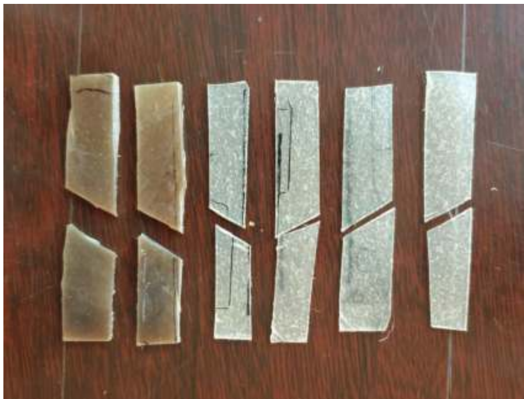
Figure (4.8): Impact test sample before and after measurement.
