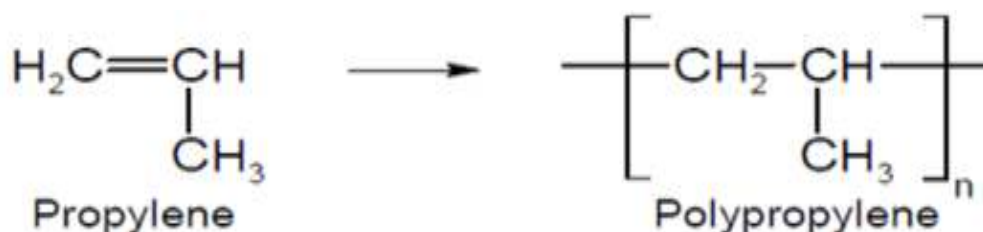
Figure (2.1): Polypropylene polymer [14]
