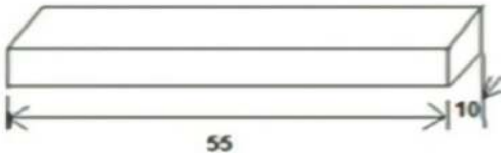
Figure (3.9): Indicate the shape of the impact sample with dimensions (ASTMD 256-87).
