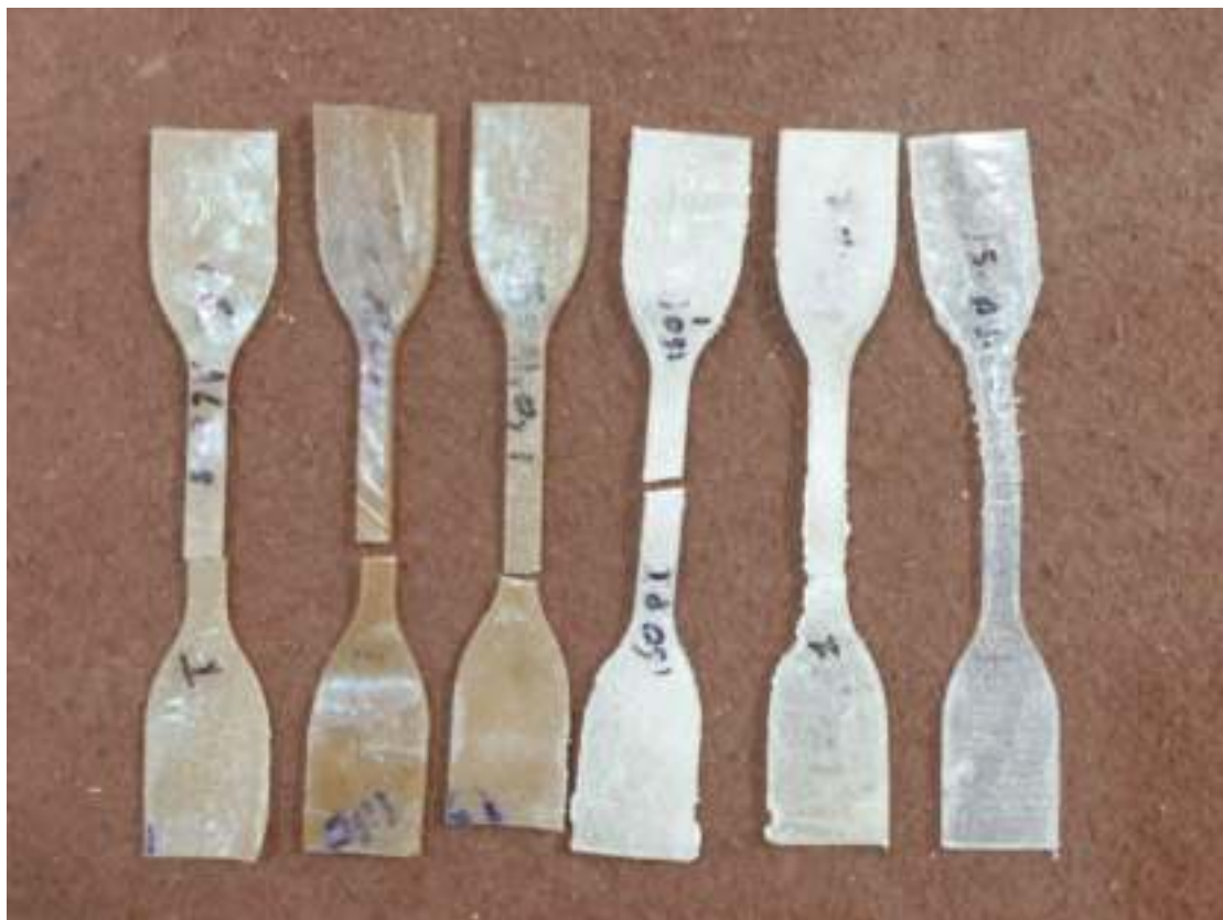
Figure (4.7): Tensile test sample before and after measurement.
