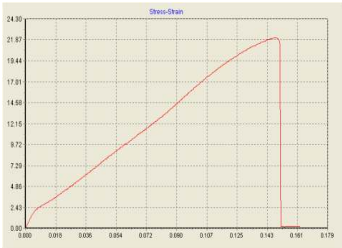
Figure (4.5): It Shows a stress-strain diagram for a sample (A5).
