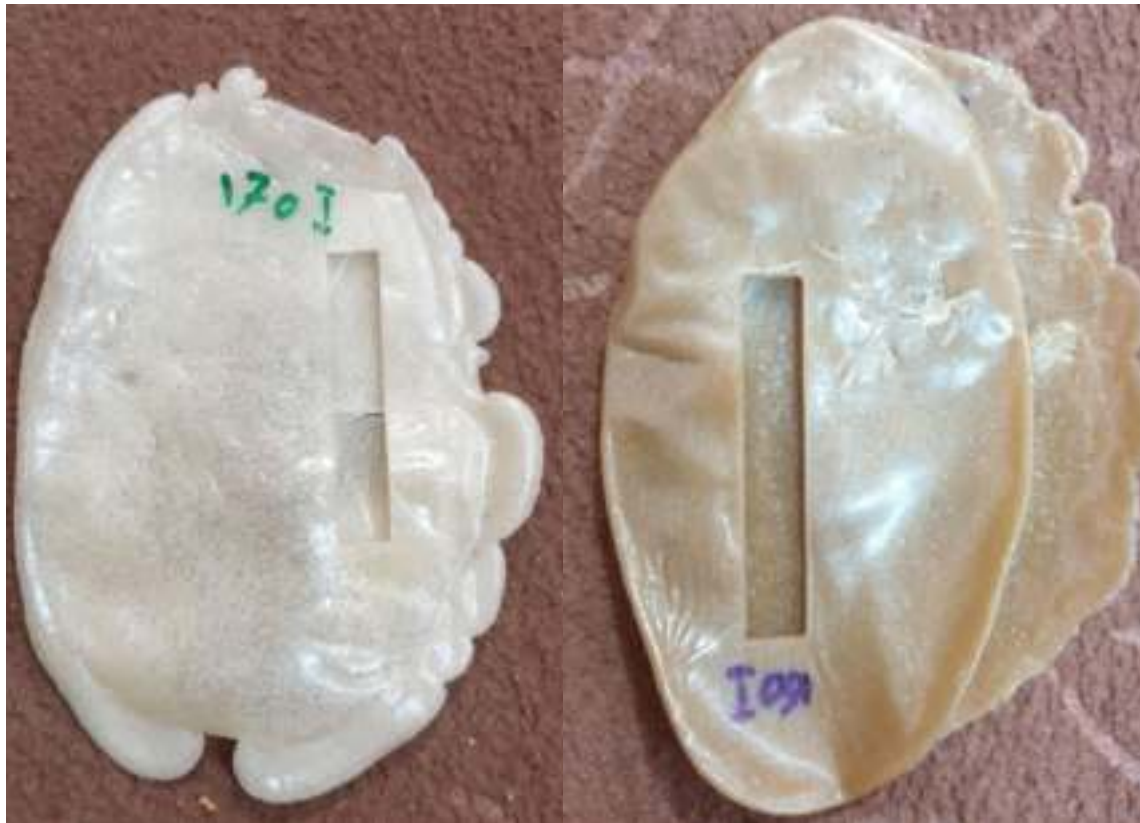
Figure (4.9): it Shaow the sheets of pure pp and PP/AL 2 O 3 for hardness test.
