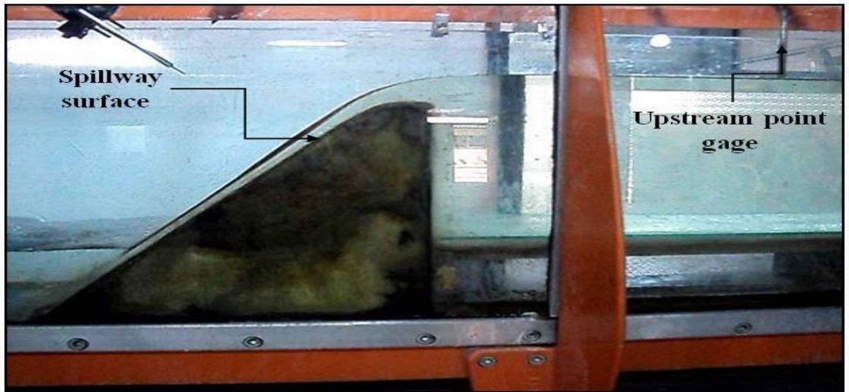
Figure 3. 4 Flow over the spillway when measuring the discharge.
