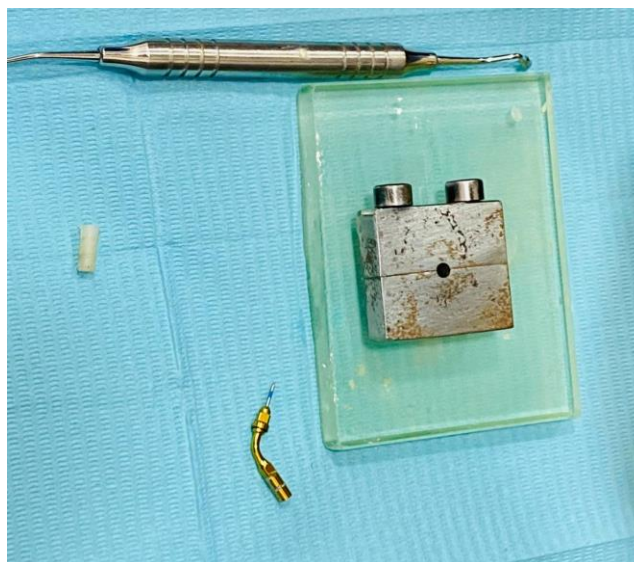
Figure (2): Position of the glass slab under the metal mold
