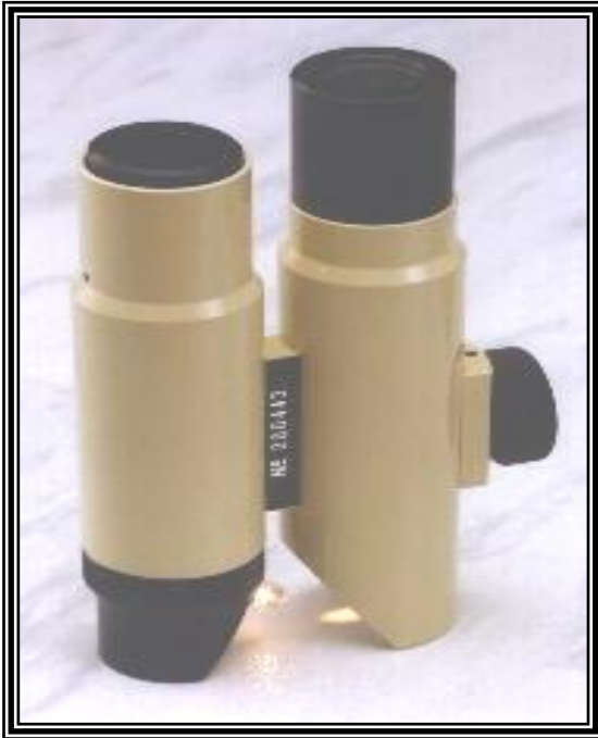
Plate ( 3 - 5): Microscope (crack width ) Plate ( 3 – 6): Measured crack width measurement
