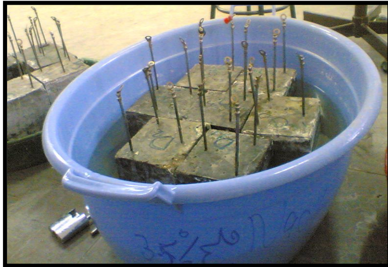
Fig.(3.8) Partial immersing of the reinforced concrete specimens in 3.5%NaCl solution
