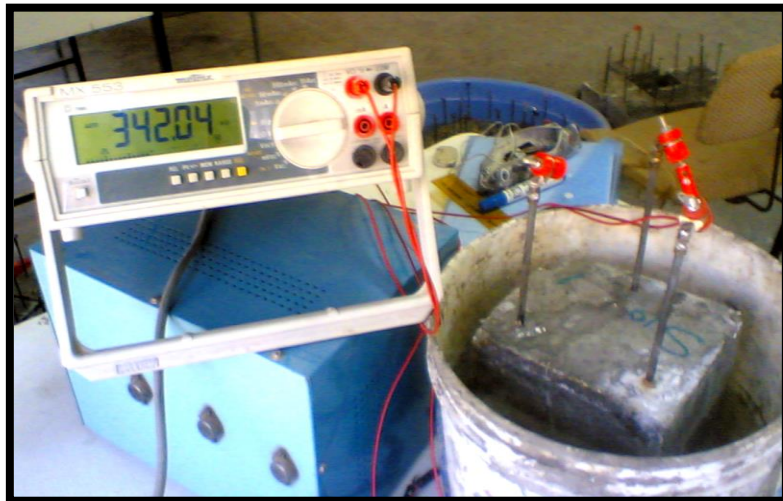
Fig. (3.9) Electrical Resistance Test for specimen with Ohmmeter
