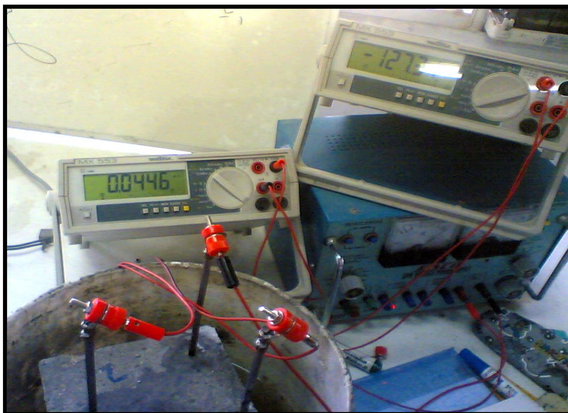
Fig. (3.12) Polarization Resistance Test Circuit.
