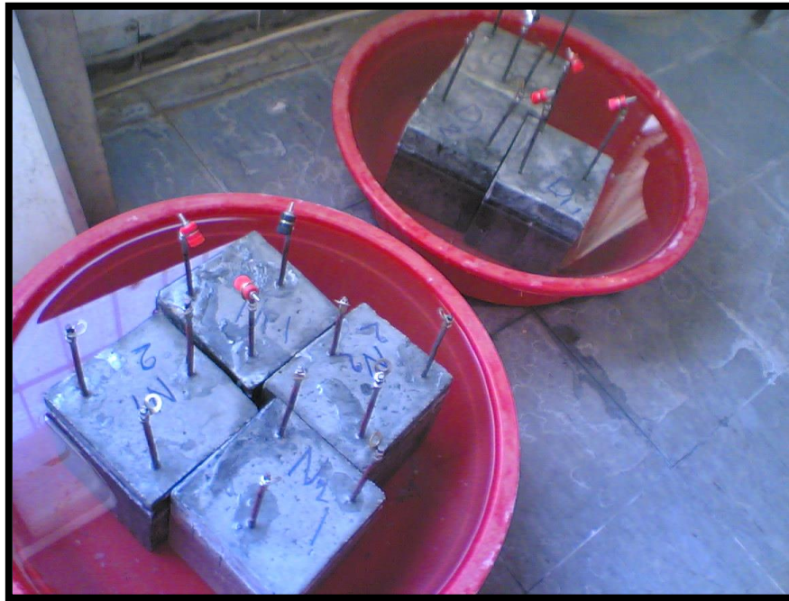
Fig. (3.6) Curing of specimens in tap water
