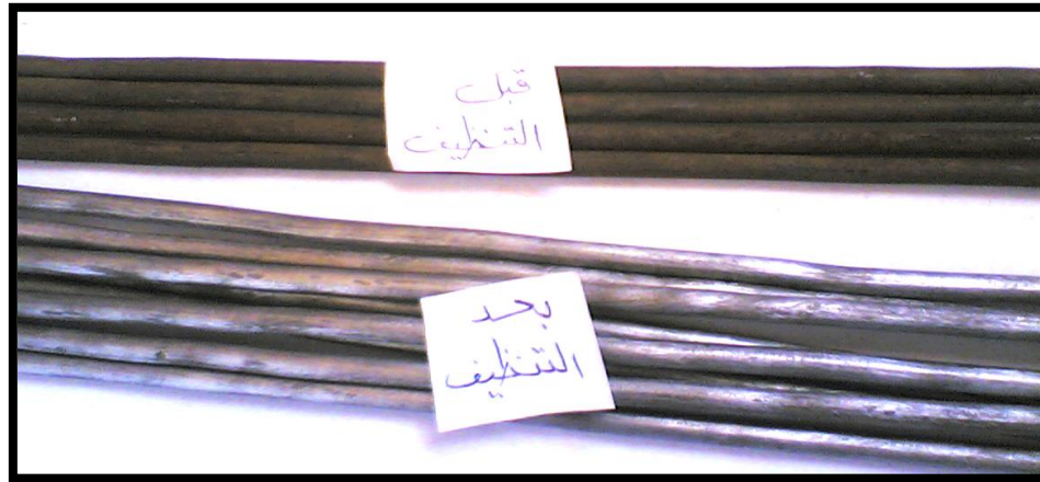
Fig. (3.5) Steel reinforced wires before and after cleaning
