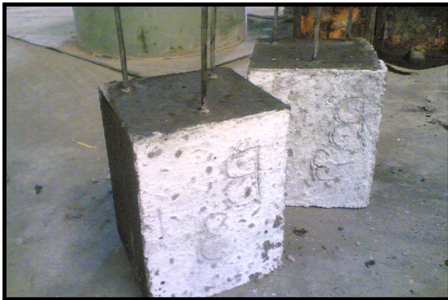
Fig. (3.2) ) The white layer on the surface of the concrete specimens due to the using of sodium benzoate admixture .
