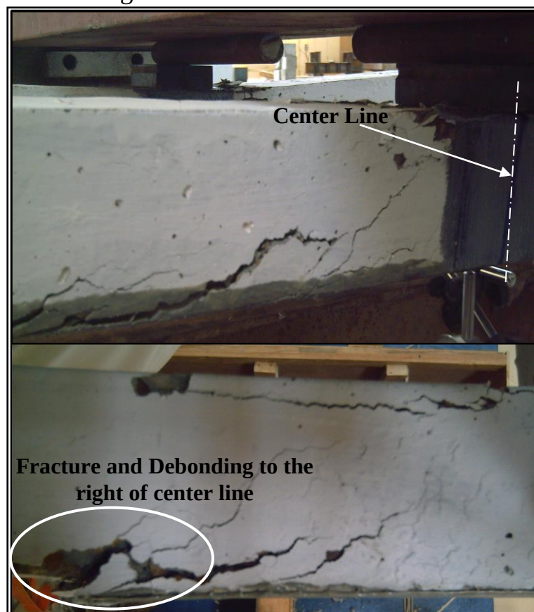
Figure (6.20) Mode of Failure for FRAME4
