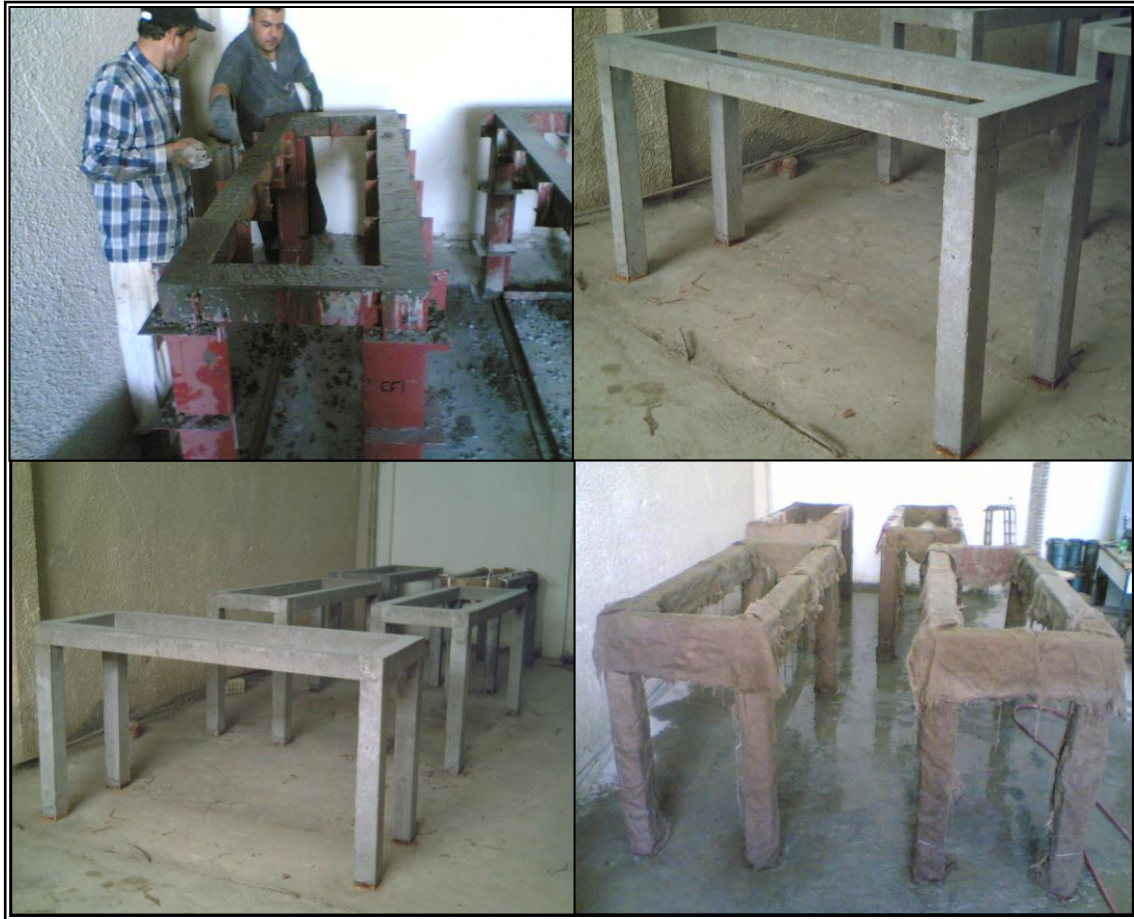
Figure (3.4) Reinforced Concrete Frames
