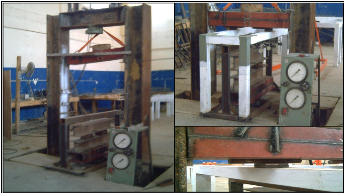
Figure (3.12) Compressive Testing Machine
