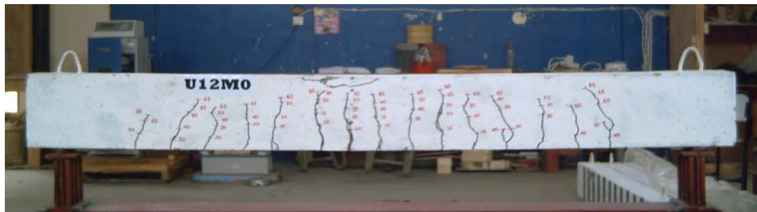
Figure 6.4: Crack pattern after failure for beam U12M0
