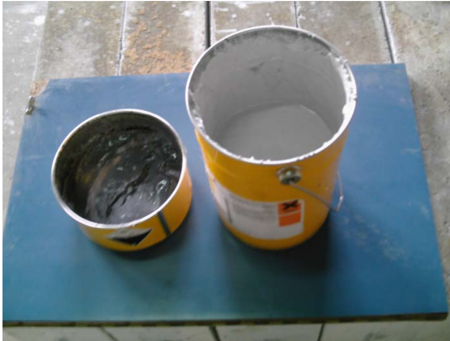
Figure 3.7: Two component epoxy adhesive
