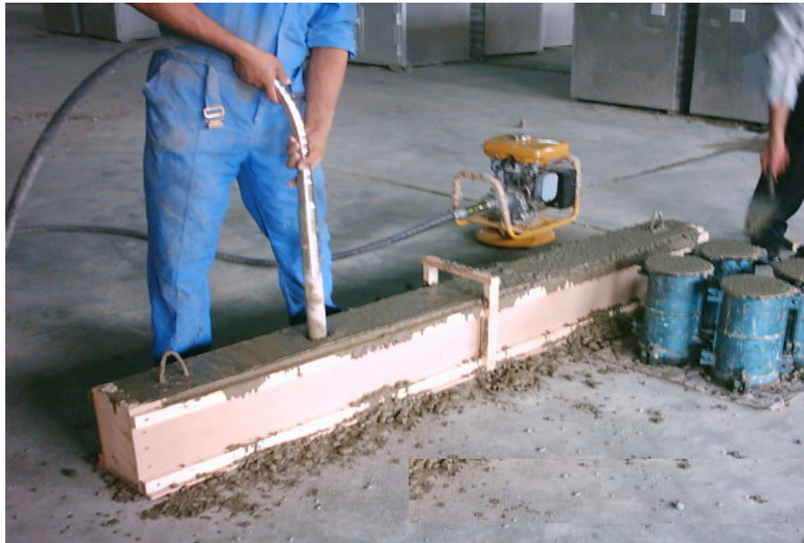
Figure 3.9: Casting beam specimens
