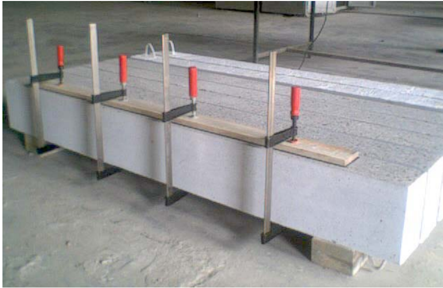
Figure 3.13: Timber packing and props to hold the CFRP plates
