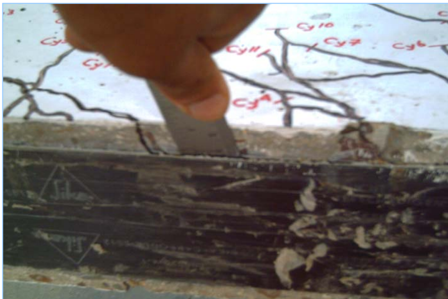
Figure 6.21: Debonding failure mode of specimen S12CE
