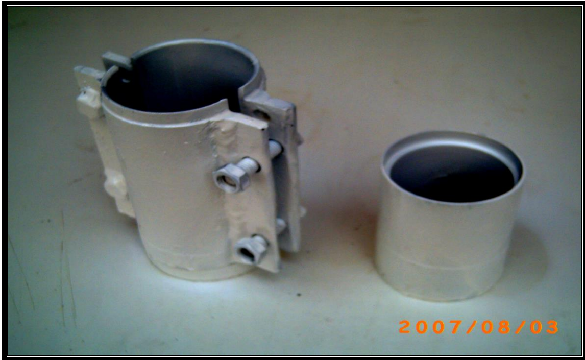
Figure (3-3) Steel split Mold and the Additional Part
