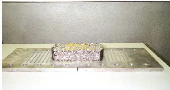
Figure 15. Test Specimen Glued to Plates.
