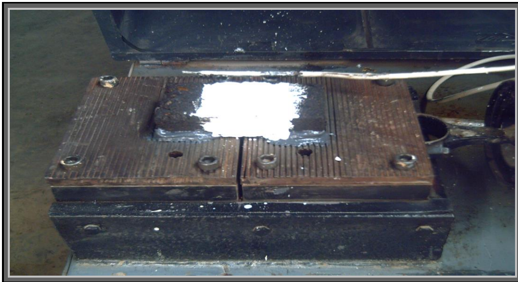
Figure (3.6) POT with Specimen Glued to the Test Plates.
