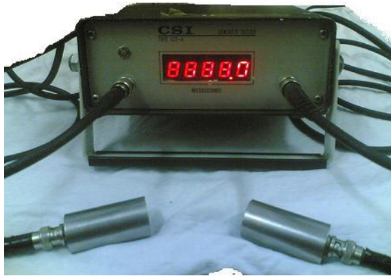
Fig (3-6) shows the configuration of Equipment of Young's Modulus of elasticity.
