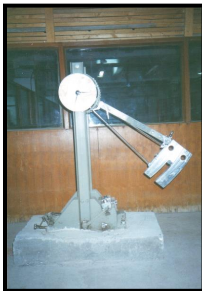
Fig (3-3) Show the Configuration of Equipment of Impact.
