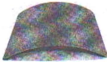
Figure (1.7): An antisymmetric laminated plate after curing
