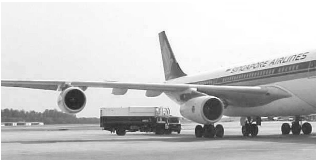
Figure (1.1): An aircraft wing idealized as a plate structure
