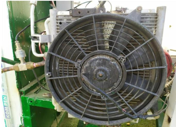
**Figure (3-6) Condenser and Fan unit**
