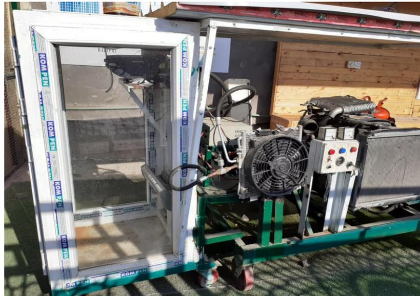
**Figure (3-4) A photograph of the parts and components of the car's cooling system and its accessories.**
