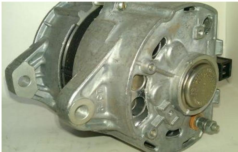
**Figure (3-2) A photograph of the Dynamo for Uaz 469 car**
