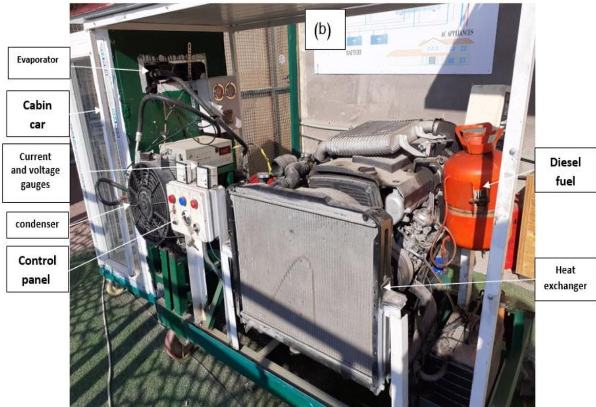
**Figure (3-1) A photograph of the proposed system with the associated measuring devices and equipment in the laboratory building at the Al-Mustaqbal University Collage (a) a back view and (b) a front view.**
