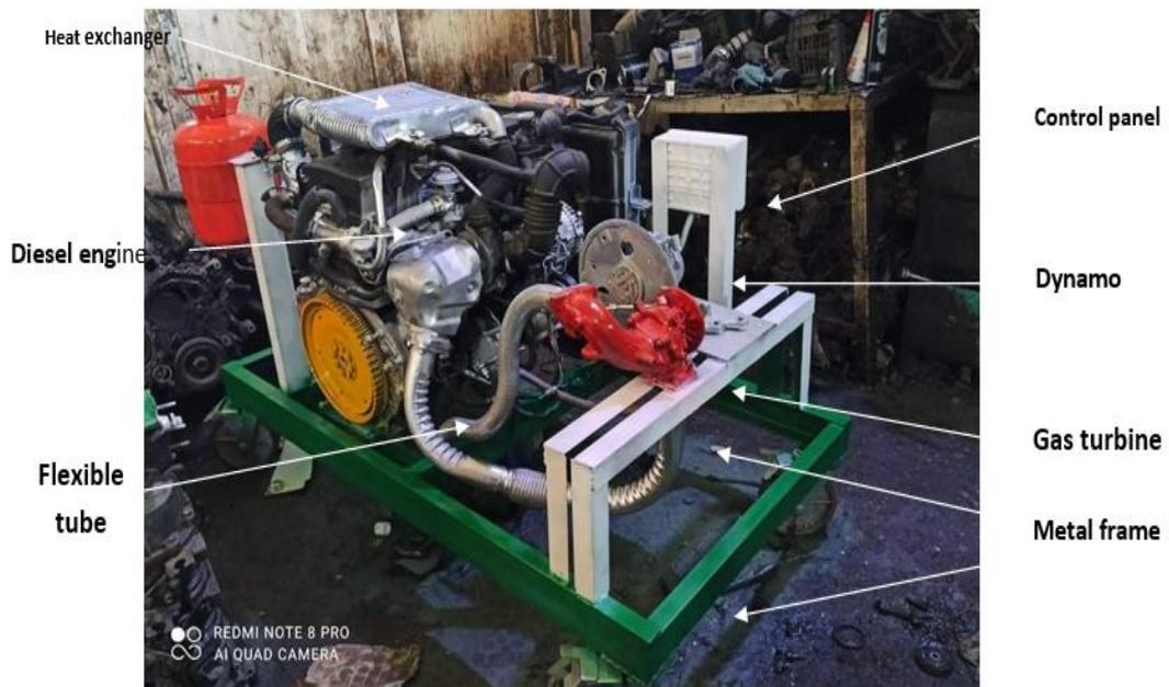
**Figure (3-3) A photograph of the main parts of the engine and its accessories**
