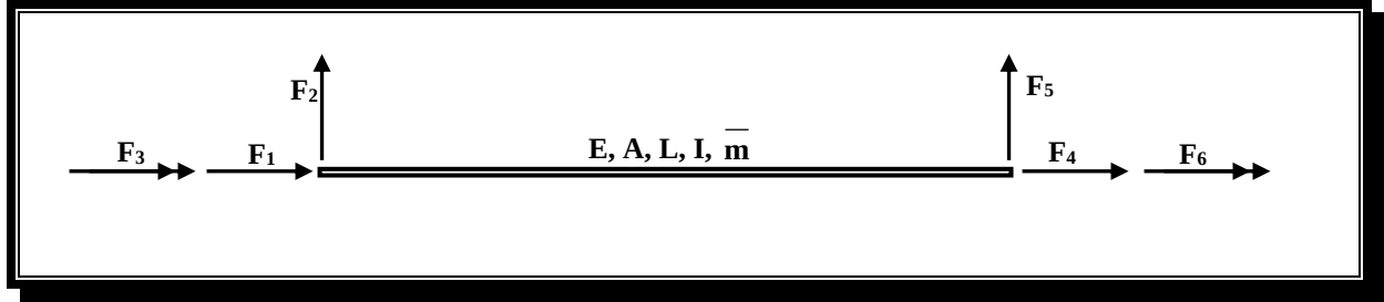
Fig.(4.1): Lumping of Mass at Element Nodes.
