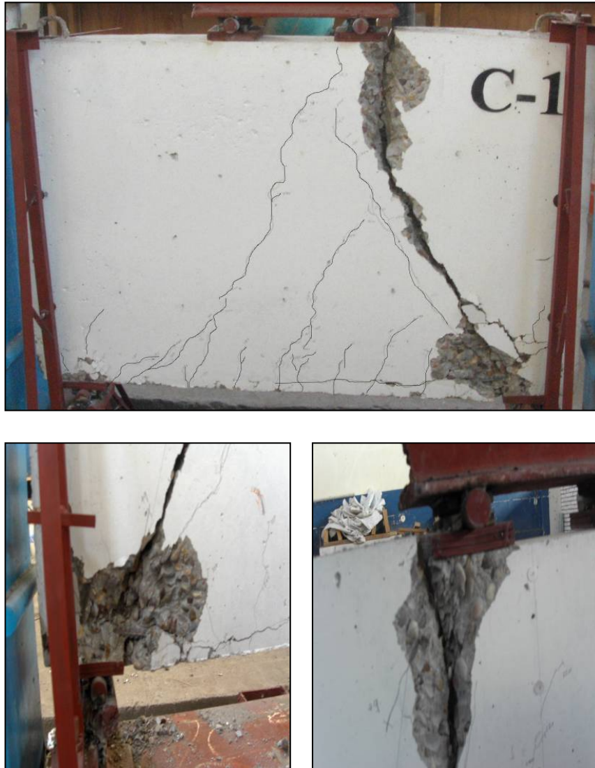
Figure 4.1 Crack pattern of beam C-1 at failure
