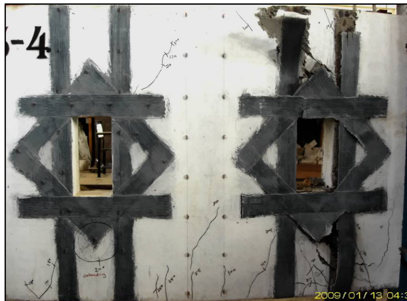
Figure 4.10 Crack patterns of specimen S-4 at failure
