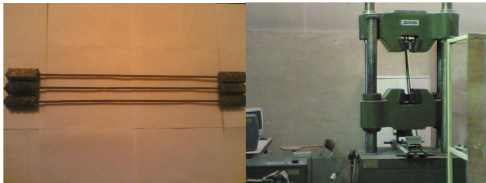
Figure (4-7): Tested steel reinforcing bar specimens and machine test.
