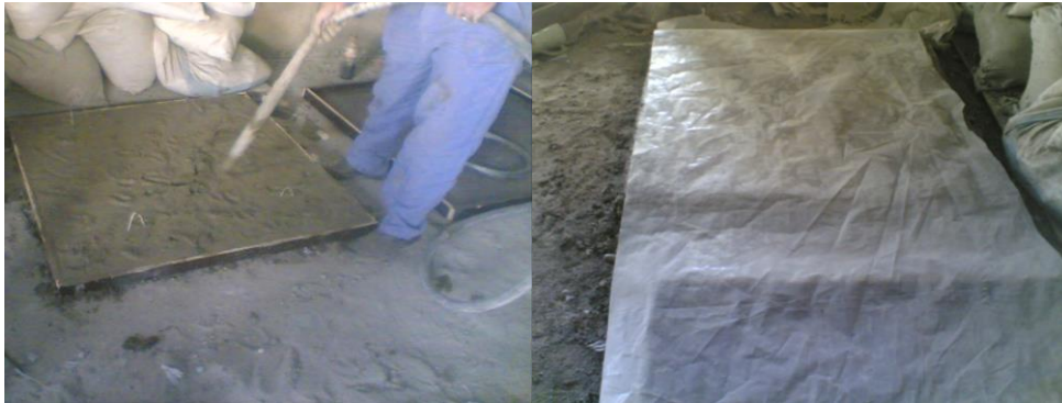
Figure (4-9): Casting and curing slab specimens.
