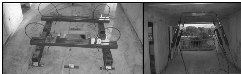
Figure (2-3): Involving cycles of loading and unloading and cross-sectional elevation of the test setup(Seliem et al., 2008).
