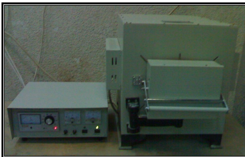
Fig. (3-17) Electrical furnace programmer by current
