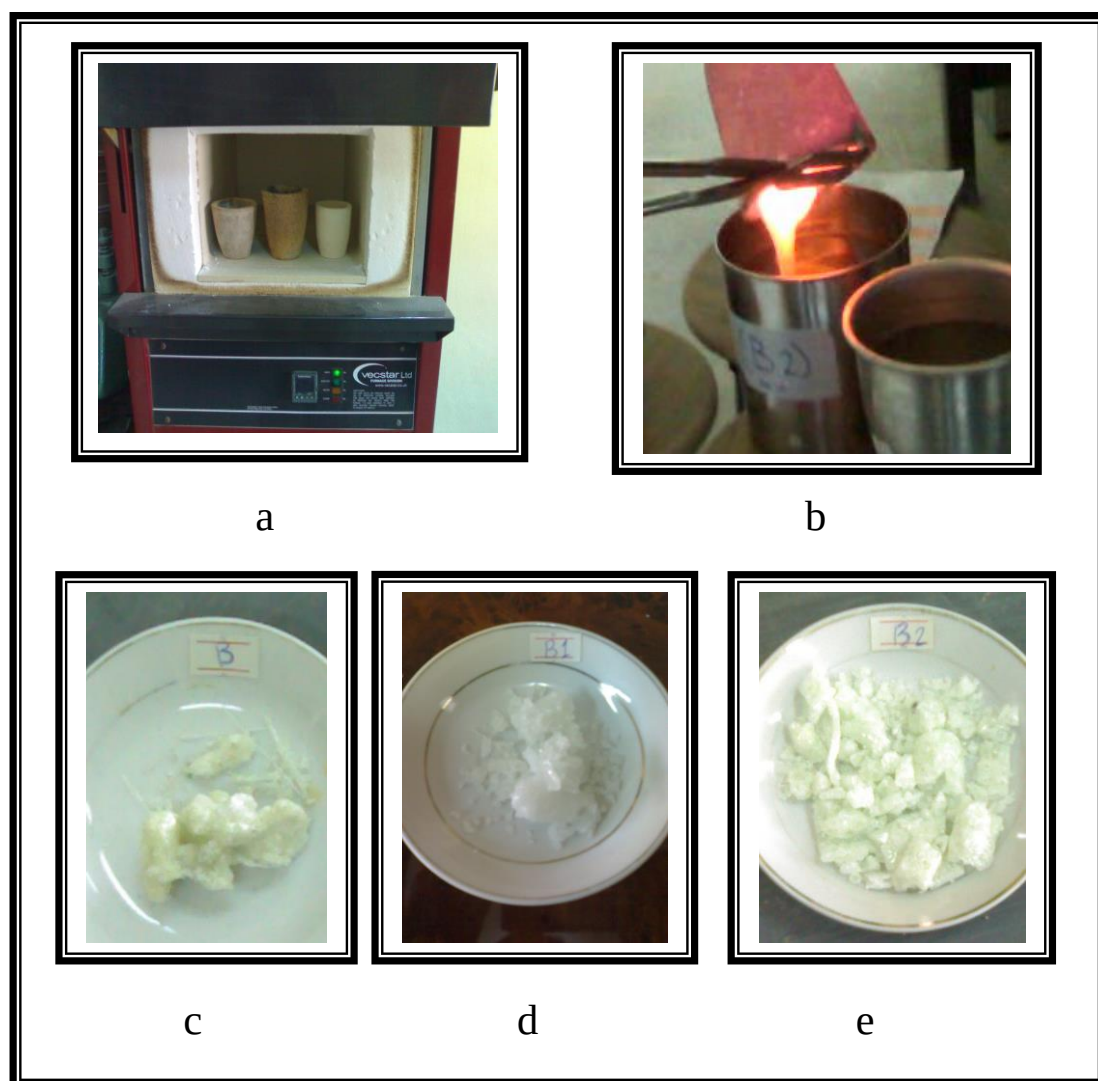
Fig. ( 3 – 8 ) a- Melting furnace b- Quenching of molten glass c- cullet of batch (B1) d- cullet of batch (B2) e- cullet of batch (B3).
