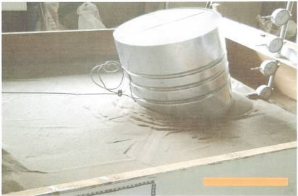
Fig.(3-19): General failure in the tested model cell.
