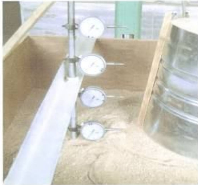
Fig. (3-15): Steel shaft carry four dial gages
