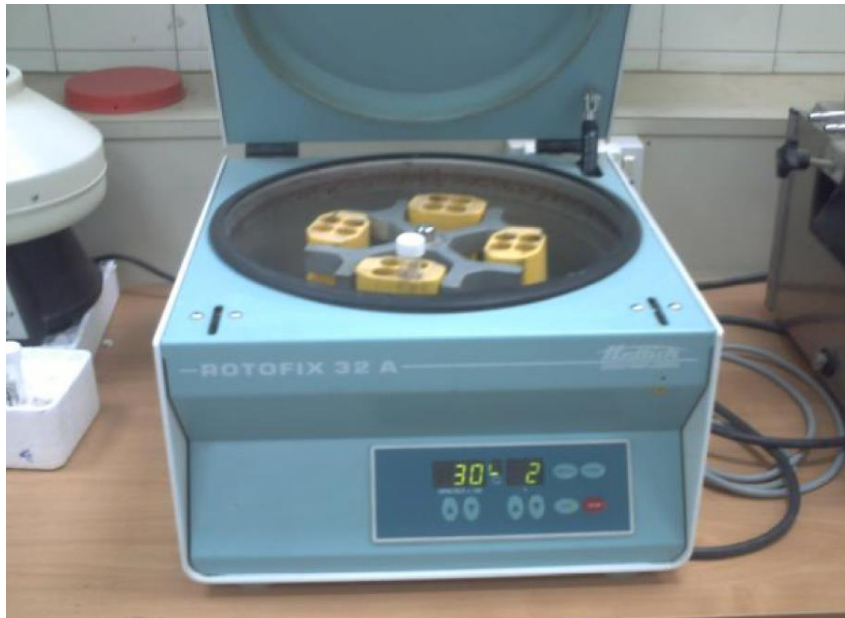
Fig.( XIII-XIII):Electronic centrifuge used for semen centrifugation and for separation of serum samples.
