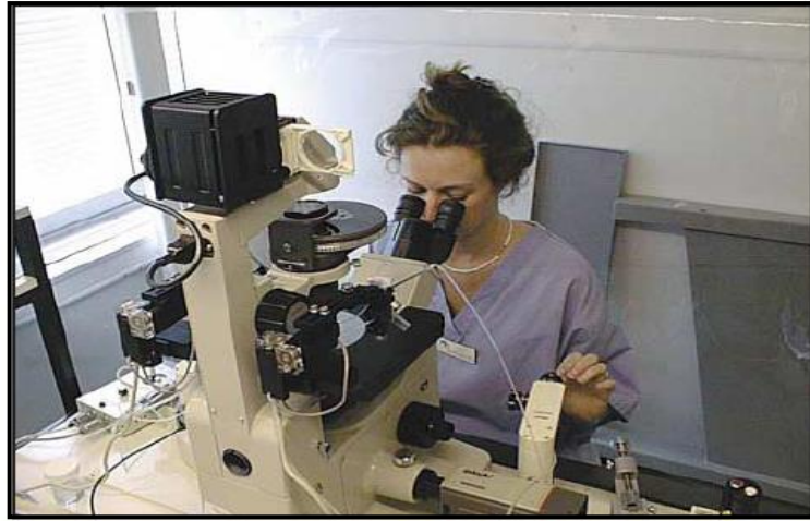
Fig(2.11) : Micromanipulation equipment required to undertake ICSI procedures. The embryologist guides the needle into the egg using joystick directed servomotors ( Braude ,2003).
